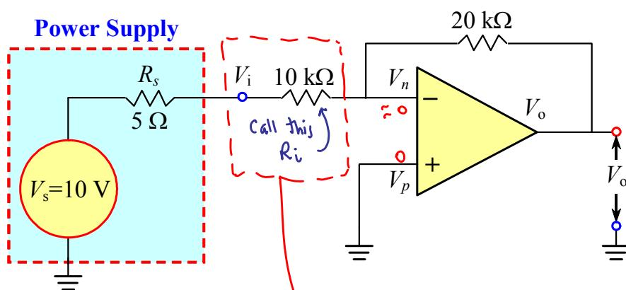
Since the input impedance of an inverting amplifier op-amp circuit is equal to  $R_1$ , the input impedance here is  $10 \text{ k}\Omega$ . Thus, the equivalent circuit (from the power supply's point of view) is:
