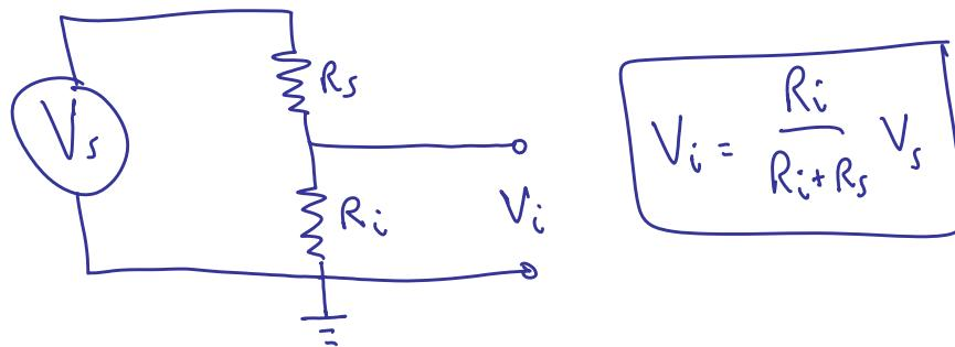
Numbers: For  $V_s = 10 \text{ V}$  ;  $R_i = R_s = 10 \text{ k}\Omega$  ;  $R_s = 5\Omega$ ,
