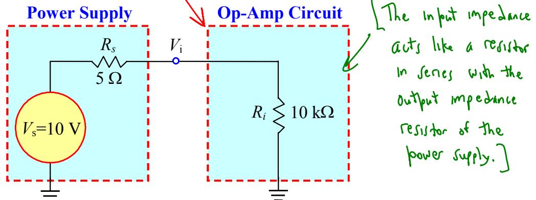
Circuit analysis — this is just a voltage divider circuit!
