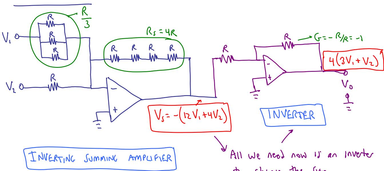
Now we are using only 2 op-amps and 10 resistors (much better than the brute force method)
