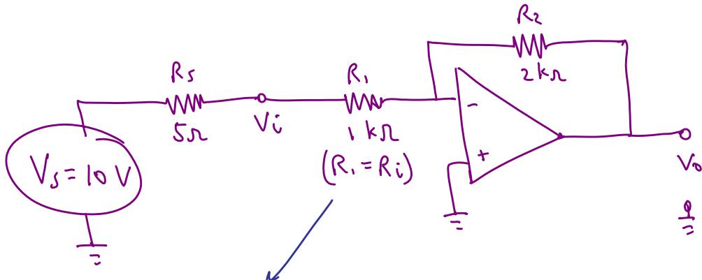
Now, the input impedance is only  $1 \text{ k}\Omega$  instead of  $10 \text{ k}\Omega$
