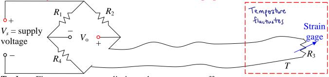
Figure out a way to eliminate the temperature effect. To do:
