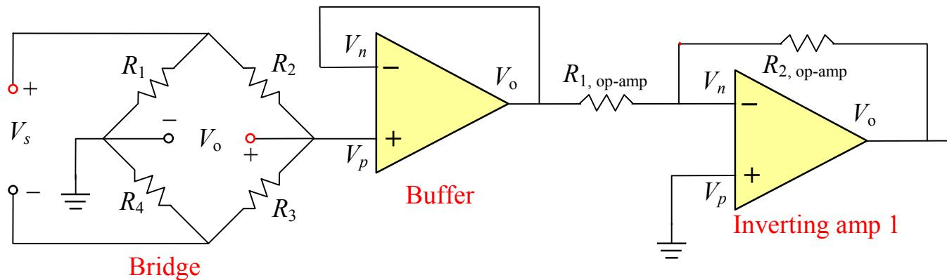
$$\begin{aligned} \text{Set } G_{\text{Stage 1}} &= G_{\text{Stage 2}} \\ &= -\sqrt{G_{\text{amp}}} = -\sqrt{1960.78} \\ &\underline{-44.281} \end{aligned}$$
