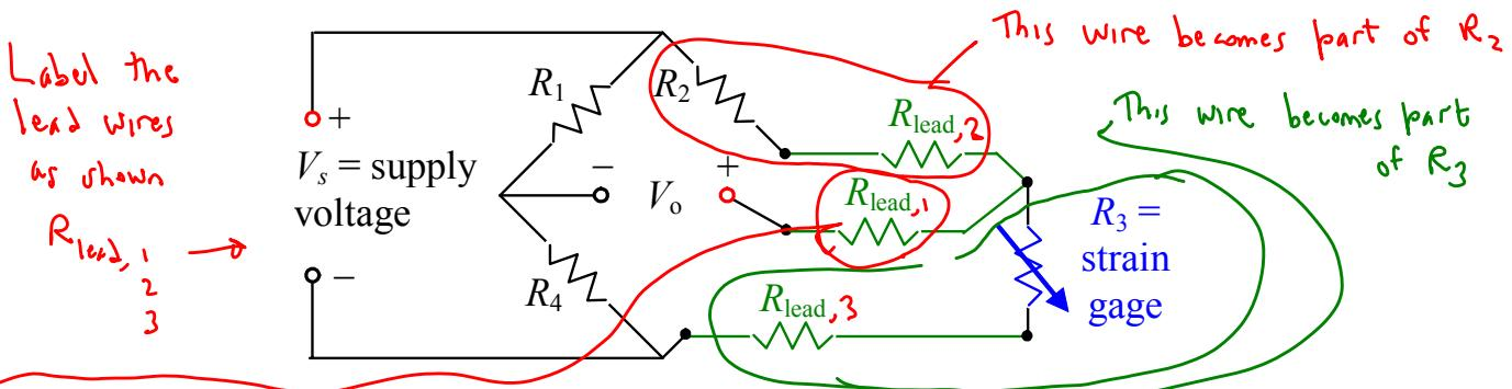
Recall the approximate equation for  $V_o$  when all four resistors of the Wheatstone bridge have small changes in resistance:
