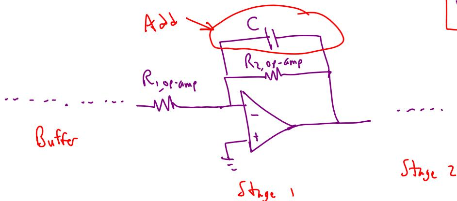
What  $C$  to use? → Since  $f_{signal} = 50 \text{ Hz}$ , let's pick  $f_{cutoff} = 150 \text{ Hz}$
