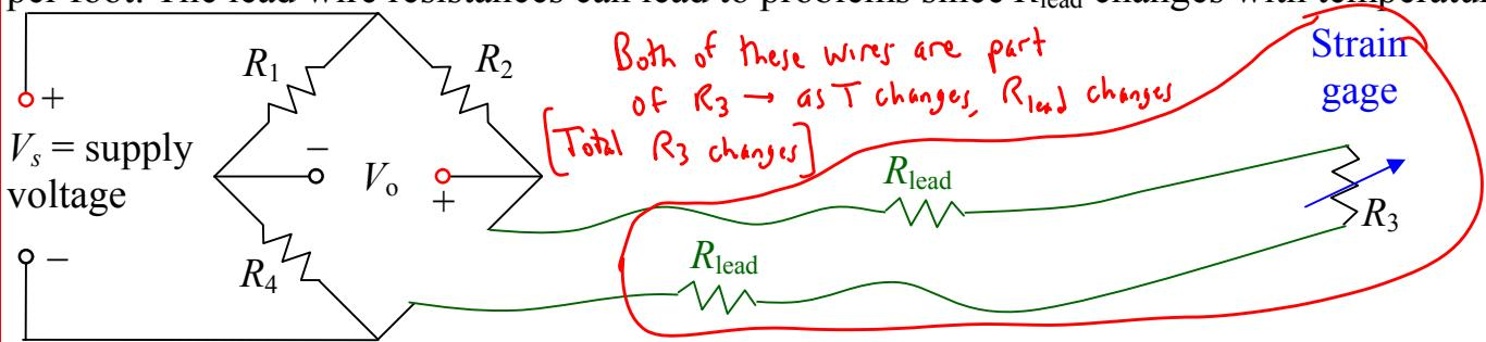
**To do:** Devise a modified circuit that will cancel out the effect of the lead wires.
