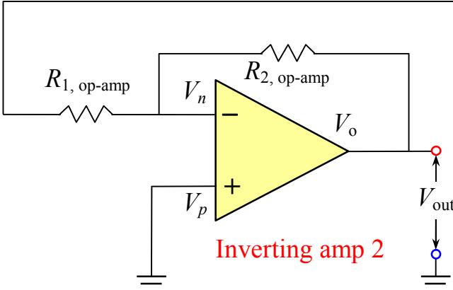
In this case, we can choose better values of the op-amp resistors. Namely, the gain of each amplifier is the square root of the total gain, i.e.,
