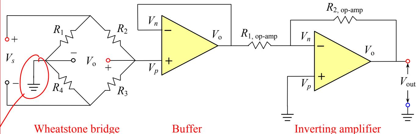
To achieve the required gain, we would use, say,  $R_{1,\text{op-amp}} = 1 \text{ k}\Omega$ , and  $R_{2,\text{op-amp}} = 1.96 \text{ M}\Omega$ .
