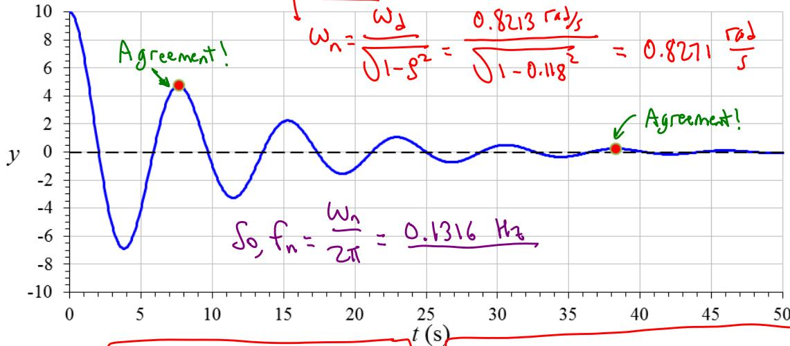
ANSWERS:  $\zeta = 0.118 = \text{damping ratio}$   $f_n = 0.132 \text{ Hz} = \text{undamped natural frequency}$
