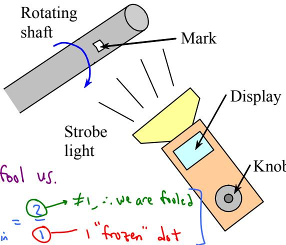
**(b) To do:** For the setup shown here, are there any strobe settings greater than 860 rpm at which the strobotachometer would give a false reading of rotation rate? Explain.
