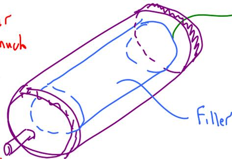
The filler cylinder is typically mounted to the (thick) end wall so it stays in place
