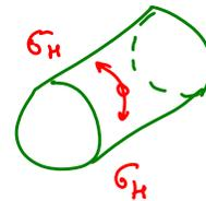
$\sigma_H$  is the one encircling the cylinder, like a "hoop"
