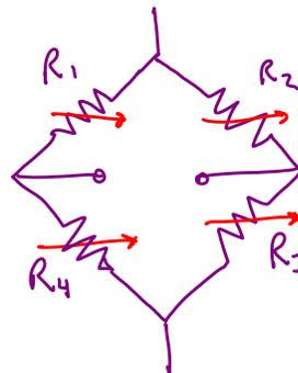
•  $R_1$  &  $R_3$  = hoop strain gages
