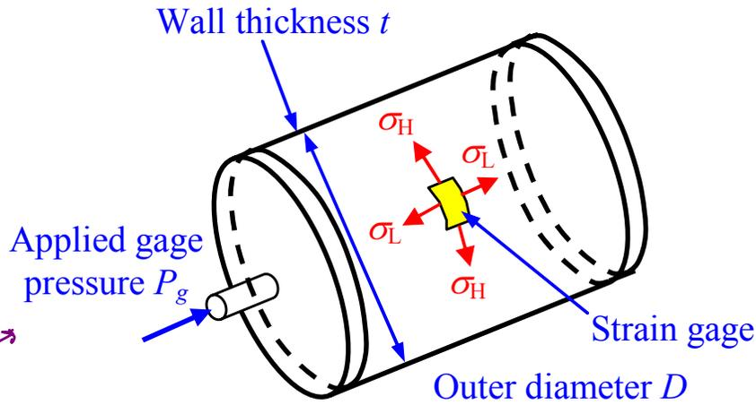
$$P_g = P_{in} - P_{atm} = \text{gage pressure being measured}$$
