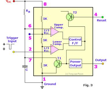
The supply current, when the output is 'high', is typically 1 milli-amp (mA) or less. The initial monostable timing accuracy is typically within 1% of its calculated value, and exhibits negligible (0.1%/V) drift with supply voltage. Thus long-term supply variations can be ignored, and the temperature variation is only 50ppm/°C (0.005%/°C).
