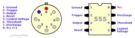
fig. 1. 8-pin T package
