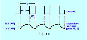
When power is first applied to the circuit, the capacitor will
