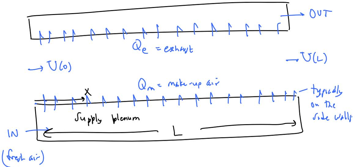
\* Balanced or Unbalanced transverse ventilation
