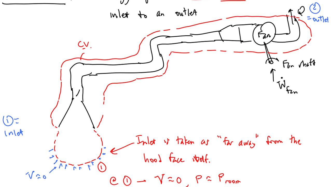
Head form of the energy eq. for Steady-State, Steady Flow (SSSF)
