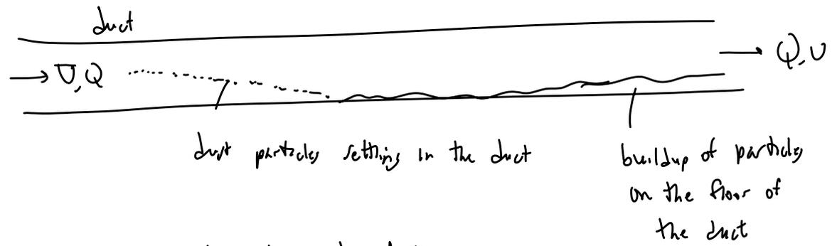
There is a minimum duct transport velocity to keep particles from settling
