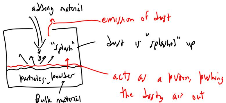
Analysis is same as with filling tank with liquid
