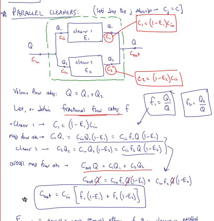
$\frac{\text{Eoverall} = \text{equivalent overall removal efficiency of these cleaners in parallel }}{\text{Eoverall} = 1 - \frac{\text{Cont}}{\text{Cin}} = 1 - \left[f_1\left(1 - E_1\right) + f_2\left(1 - E_2\right)\right]}$  In parallel
