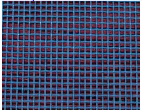
Example of a woven filter, where the woven "threads" are very tight and do the actual filtering; this one is *metal* (from <a href="http://www.ap-by.com/?Product105/xxw.html">http://www.ap-by.com/?Product105/xxw.html</a> ):
