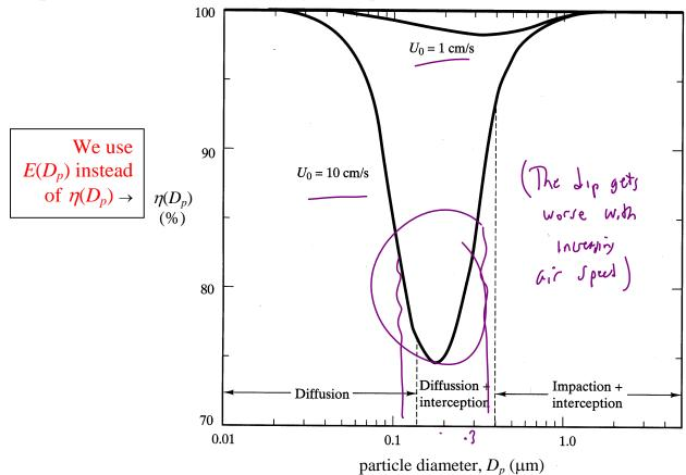
Filter grade efficiency for two face velocities; filter thickness H = 1.0 mm, solids fraction  $f_f = 0.05$  (porosity  $\varepsilon = 0.95$ ), single fiber diameter  $D_f = 2$  µm (adapted from Hinds, 1982).
