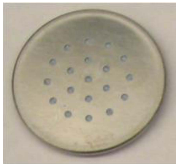
Figure 1. (Color online) Picture of a Li/air cell (type 2325) with multiple air diffusion holes.
