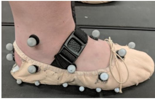
Fig. 2: Modified ballet slipper for second part of study, foot markers, and foot plate markers (three-quarter plate shown).
