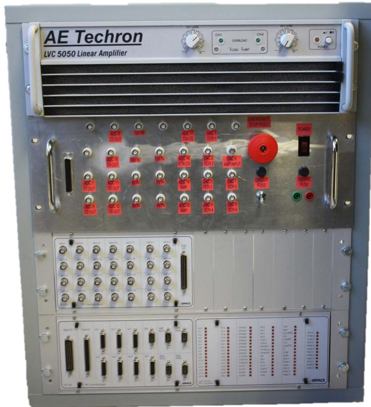
**Figure A.1.** The PBTM is shown below the amplifier and above the DAQ system.
