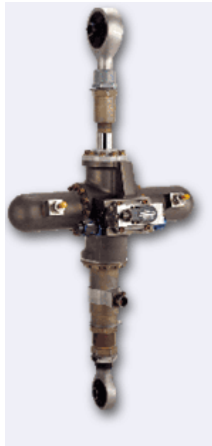
Figure 4.3: UH-60 Hydraulic Pitch Link [41].
