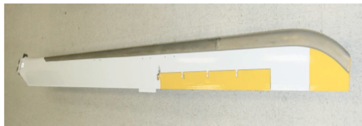
Figure 1.3. Rotor Blade with Trailing Edge Flap Developed by the Boeing Co. [14]
