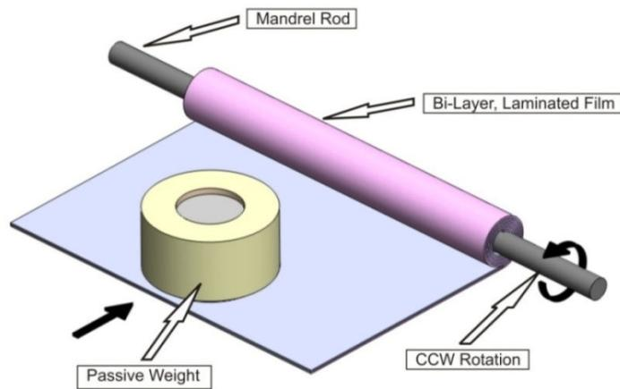
**Figure 3-21: Rolling Step Illustration Using the Weight**
