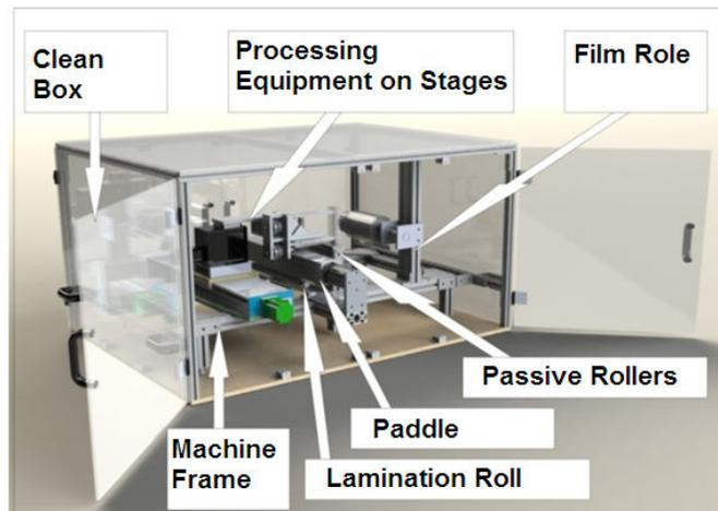
**Figure 2-4: SolidWorks Rendering of Actuator Fabrication Machine**
