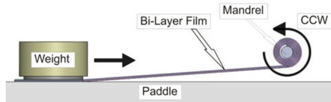
**Figure 3-1: Rolling Operation Illustration**
