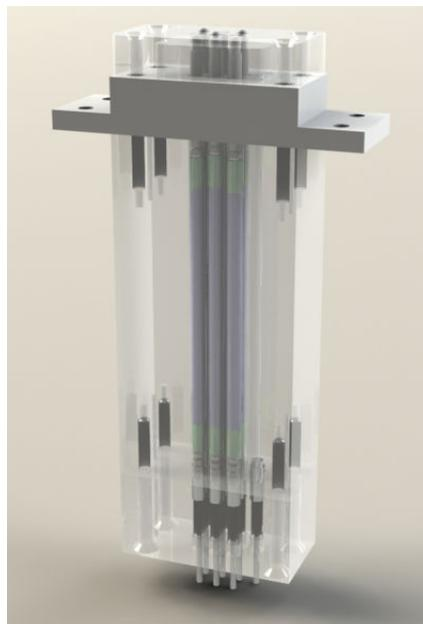
**Figure 4-8: SolidWorks Rendering of Braille Cell under Production**
