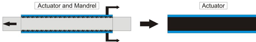
**Figure 3-19: Low Shear Force for Actuator Removal**
