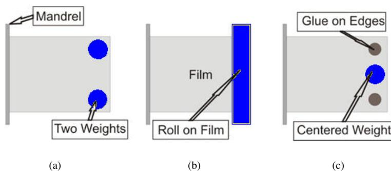
**Figure 3-20: (a) Experiment 1, Weights at Opposite Edges (b) Experiment 2, Roll Across Edge (c) Experiment 3, Weight centered on Edge**
