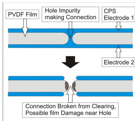
**Figure 3-13: Film Clearing Illustration**
