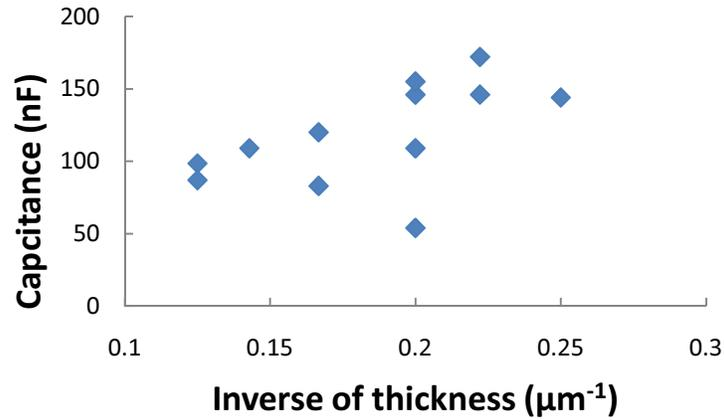
Figure 3-10: Measured Capacitance with Varying Film Thickness, 1.25-1.5 mL Electrode Applications
