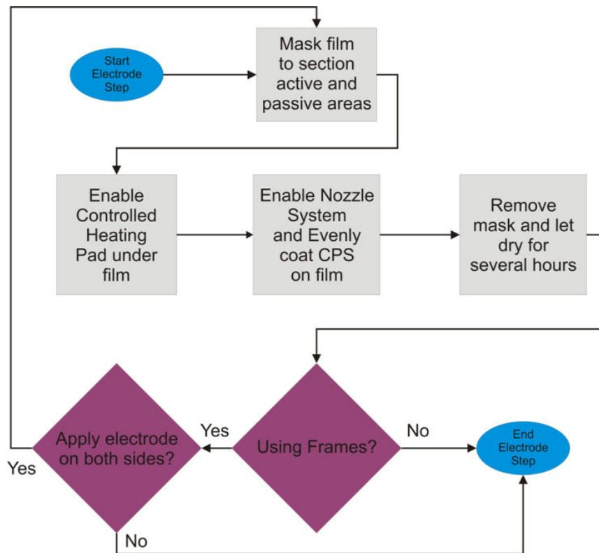
Figure 3-12: Electroding Step Using Frame Manufacturing Flow Chart
