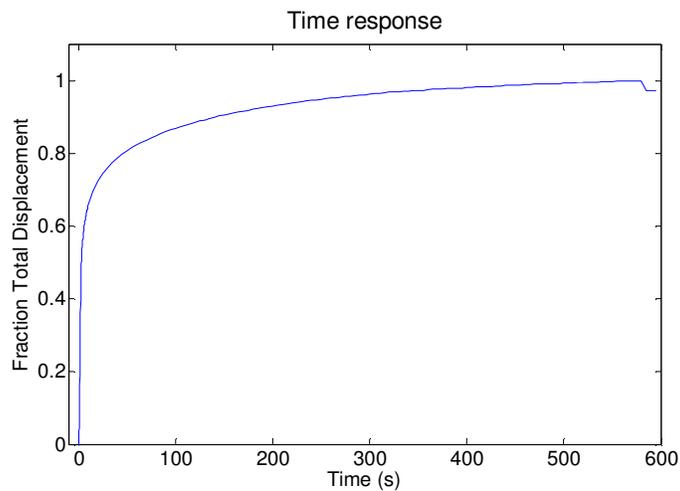
**Figure 4-4: Response Time of PVDF Tube Actuator**
