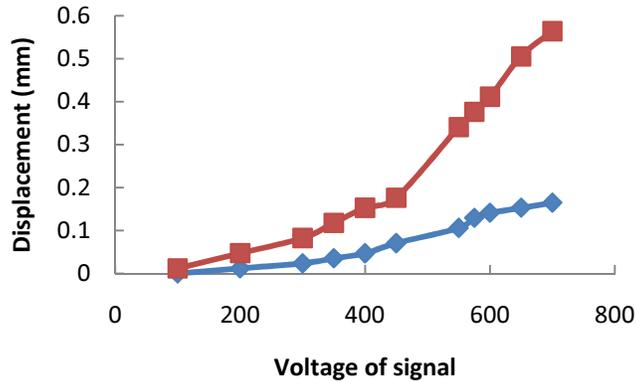
**Figure 4-3: Actuator Drifting From 0.1 Hz Sine Signal (square) Active (diamond) Inactive**
