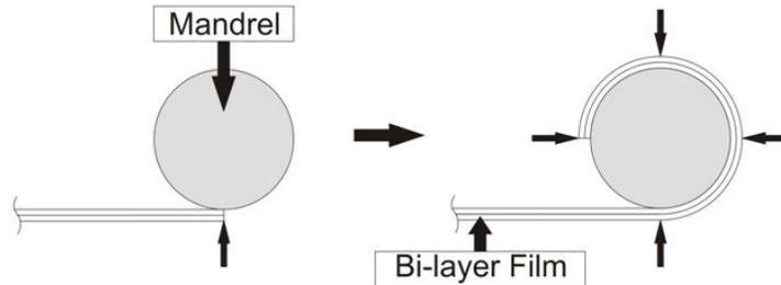
**Figure 3-18: High Normal Force for Bi-Layer Film Rolling**
