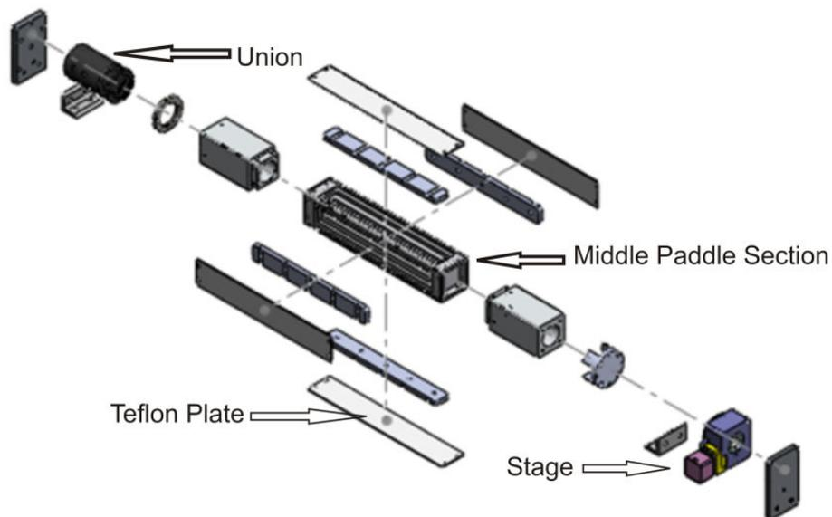
**Figure 2-8: Exploded View of Paddle Assembly**
