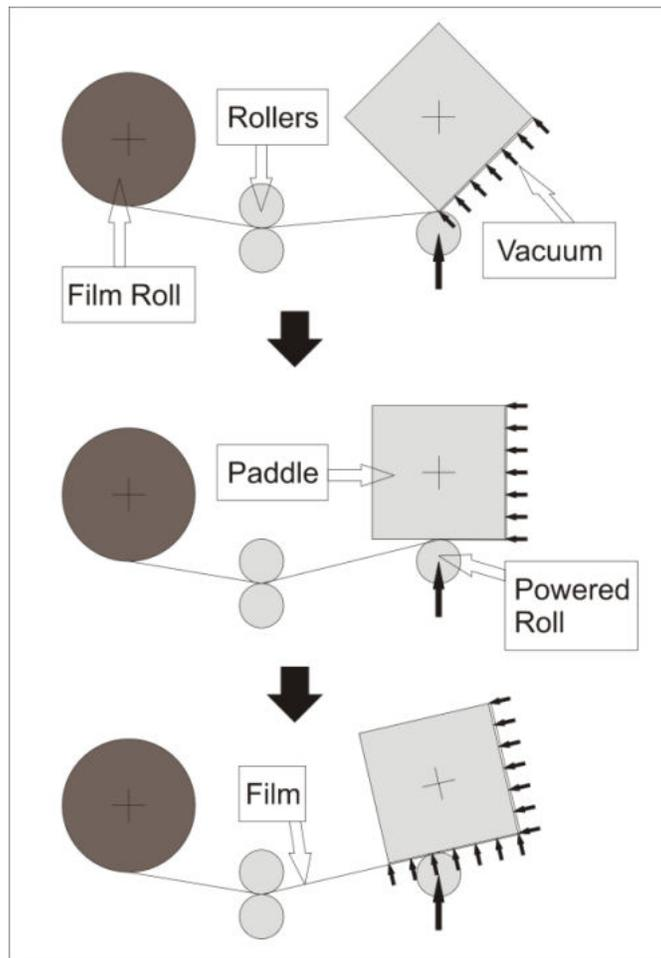
**Figure 2-10: Film Roll Manufacturing - Film Handling Illustration**
