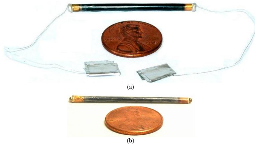
**Figure 3-26: (a) Actuator with Wire Leads (b) Actuator with Steel Ball Ends**
