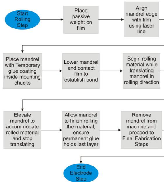
**Figure 3-23: Flow Chart for Rolling Operation**
