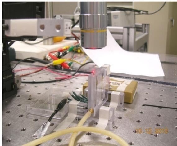
**Figure 4-5: Laser Vibrometer Testing Apparatus**
