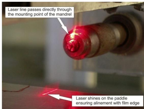
**Figure 3-24: Laser Line Projecting Mandrel Location on Paddle**
