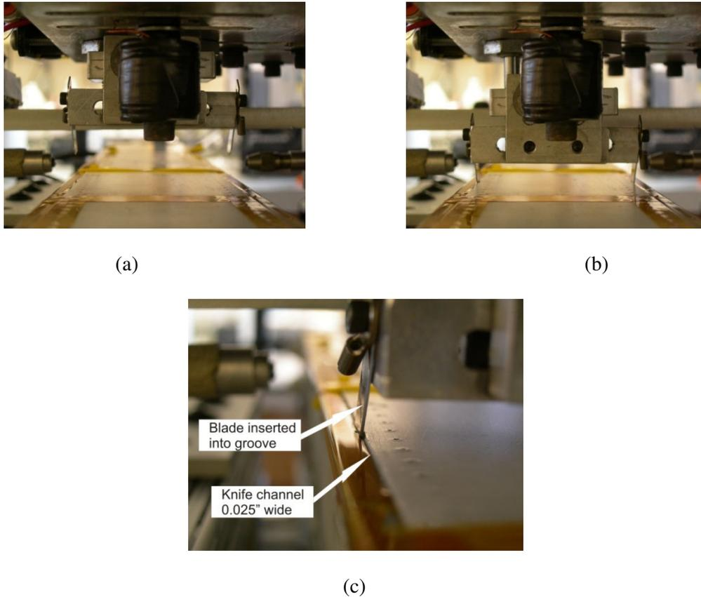
**Figure 3-17: (a) Knife Assembly Disengaged (b) Knife Assembly Engaged (c) Close Up Of Knife Assembly in Paddle Groove**
