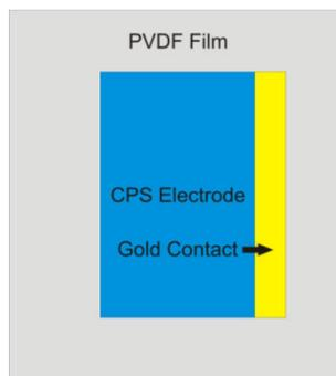
**Figure 3-6: Gold Sputtered On CPS Edge for Better Electrical Connection**
