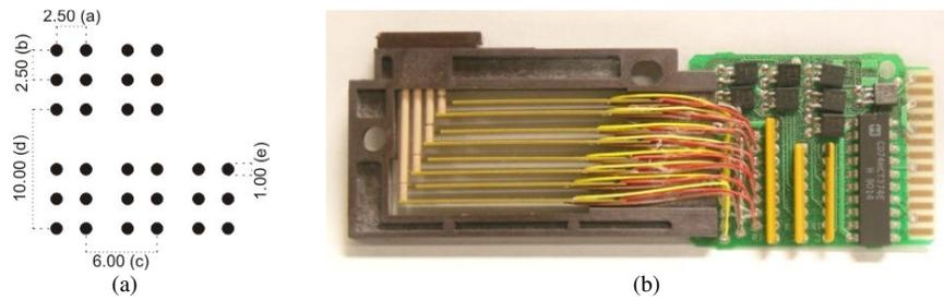
**Figure 1-1: (a) Braille Cell Dimensions in mm (b) Braille Cell from Commercially Available Display**
