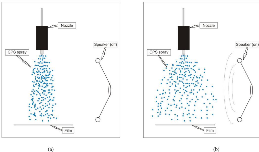
**Figure 3-4: (a) CPS Diffusion with Nozzle Only (b) CPS Diffusion Accelerated with Speaker System**
