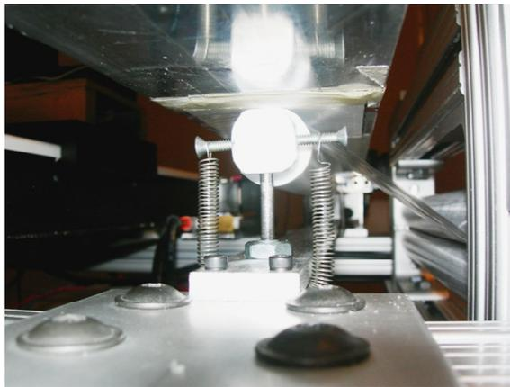
**Figure 3-15: Continuous Lamination from Film Roll**
