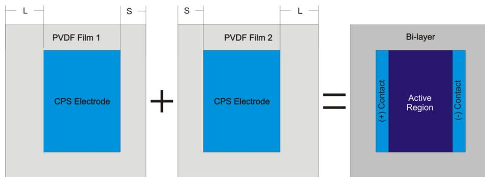
**Figure 3-5: Electrode Orientation for Active and Inactive Electrode Areas**
