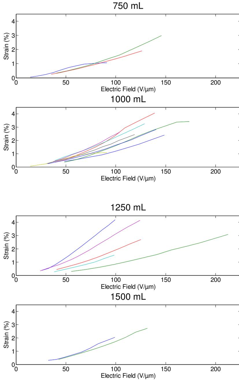
A-Figure C-1: Strain versus Electric Field Plotted by Electrode Thickness
