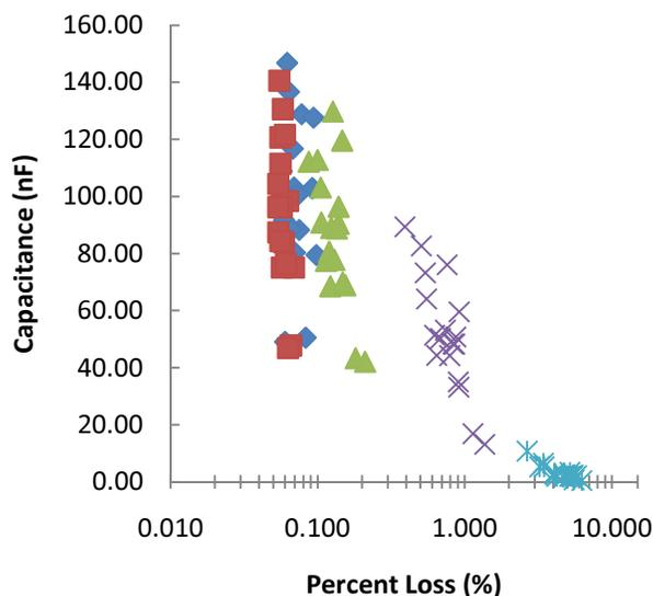
**Figure 3-7: Loss and Capacitance Results for CPS Electrode (diamond) 20 Hz (square) 100 Hz (triangle) 1KHz (cross) 10 KHz (star) 100 KHz**
