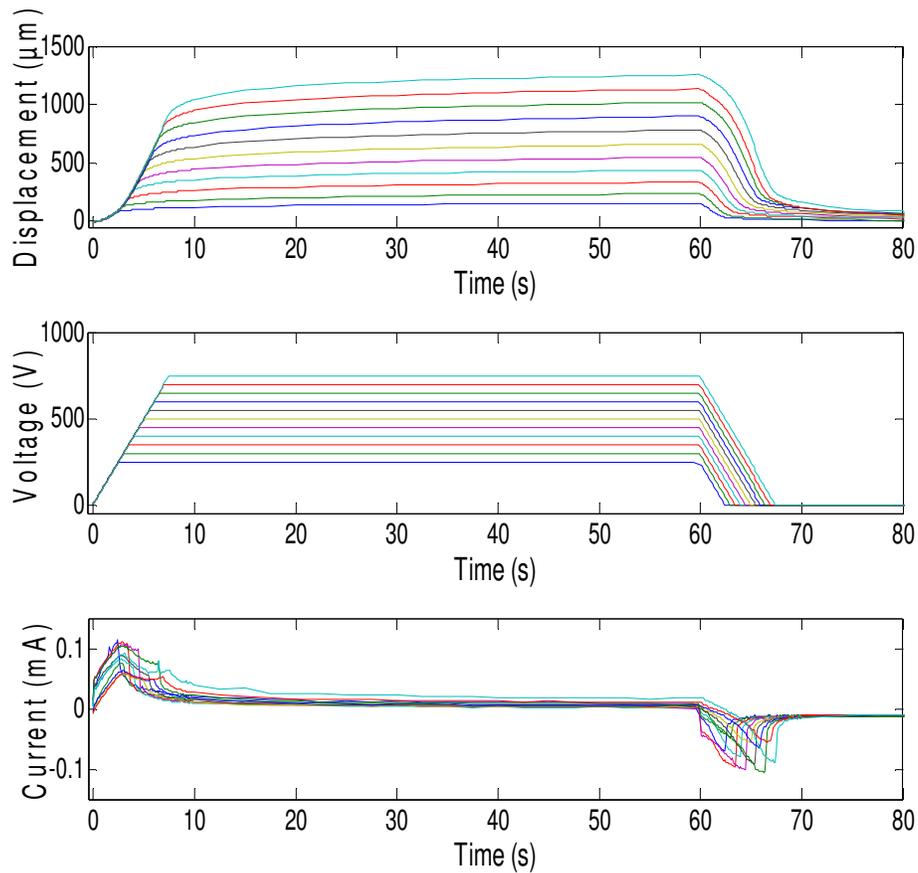
**Figure 4-6: Actuator Displacement, Applied Voltage and Current with 50 V Incremental Voltage from 200V-750V versus Time**
