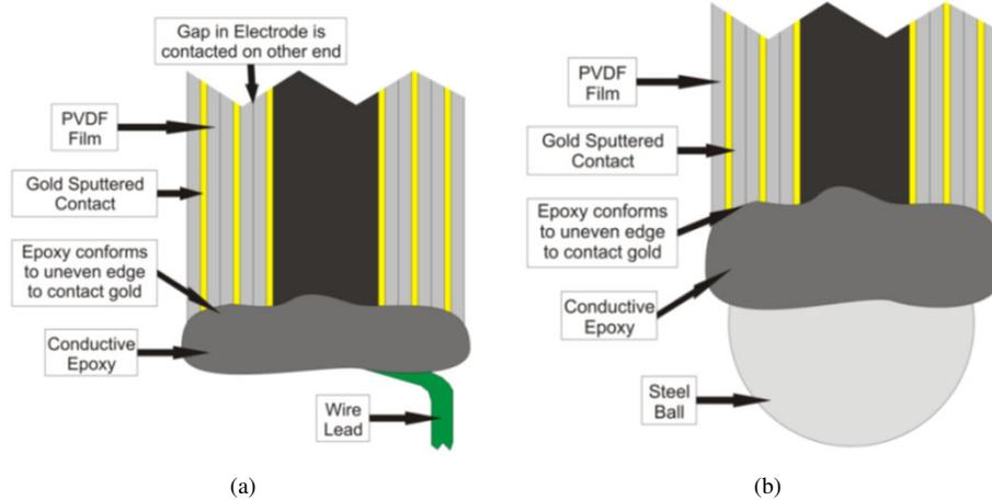
**Figure 3-25: (a) Actuator End with Wire Leads (b) Actuator End with Steel Balls Attached**
