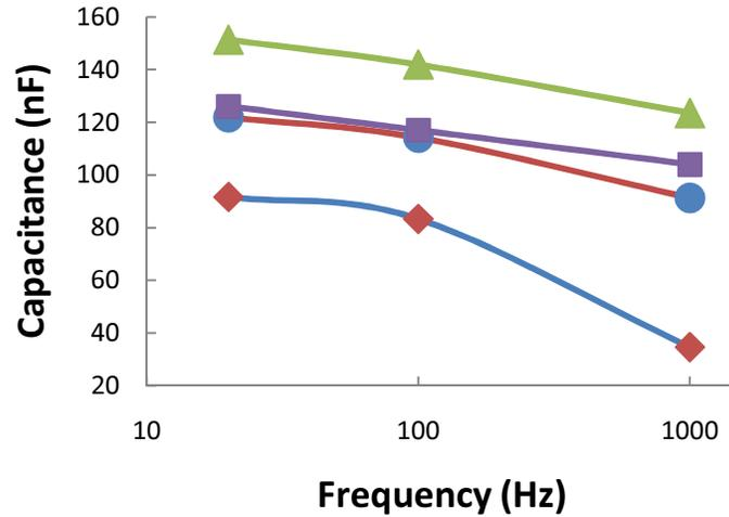
Figure 3-8: Average Capacitance for Electroding Application (diamond) 0.75 ml (circle) 1 ml (triangle) 1.25 ml (square) 1.5ml
