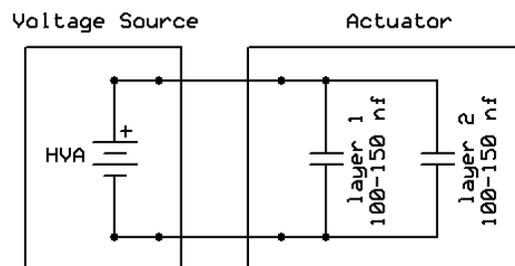
**Figure 2-2: Schematic of Individual Bi-Layer Actuator with Estimated Capacitance**
