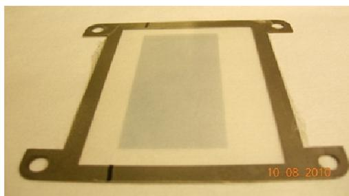
**Figure 3-3: Electrode PVDF Sample**
