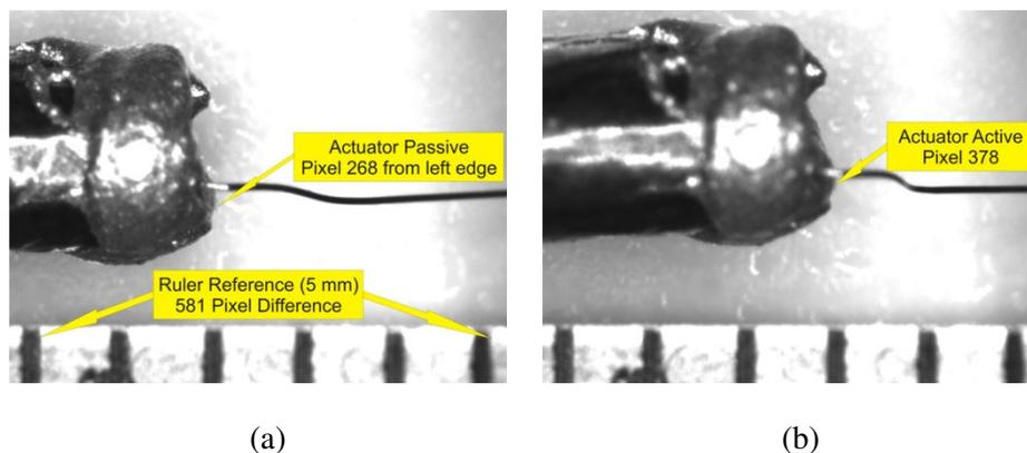
**Figure 4-1: Camera Showing Actuator Currently Passive (b) Camera showing Actuator Charged to 600V**
