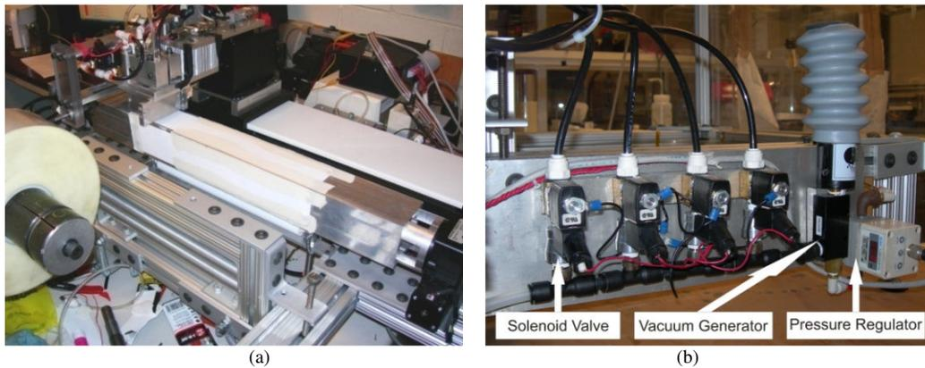
**Figure 2-7: (a) Paddle Assembly (film working surface) (b) Vacuum System**
