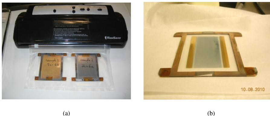
**Figure 3-16: (a) Frame Lamination Using Vacuum Bags (b) Laminated Bi-Layer PVDF Sample**
