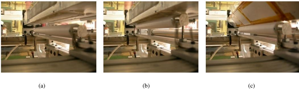
**Figure 2-9: (a) Lamination Roll Disengaged (b) Lamination Roll Engaged (c) Lamination Roll on Paddle Corner**
