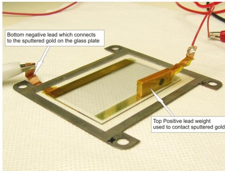
**Figure 3-14: Clearing and Capacitance Measuring Apparatus with Film Sample**
