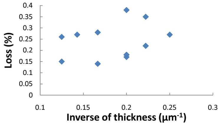
Figure 3-11: Measured Loss with Varying Film Thickness, 1.25-1.5 mL Electrode Applications
