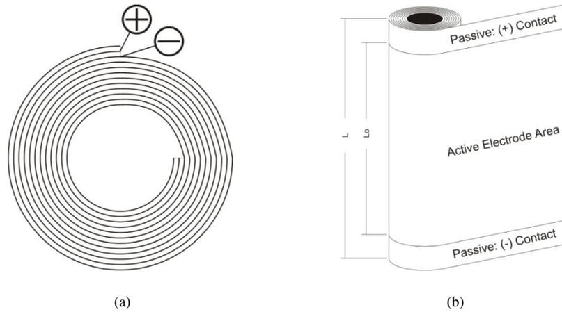
**Figure 2-3: (a) Cross-Section of Bi-Layer Actuator (b) Actuator Profile with Active/Passive and Electrical Areas Indicated**
