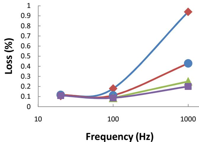
Figure 3-9: Average Loss for Electroding Application - (diamond) 0.75 ml (circle) 1 ml (triangle) 1.25 ml (square) 1.5 ml
