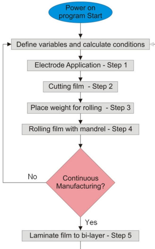
Figure 3-28: Major Operation Flow Chart of Machine Algorithm
