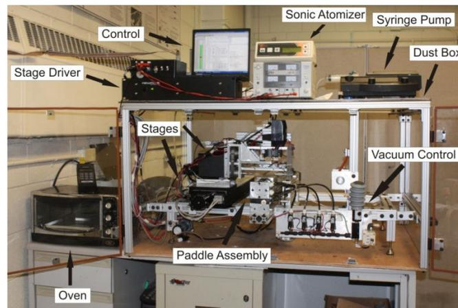
**Figure 2-5: Photograph of Actuator Fabrication Machine**
