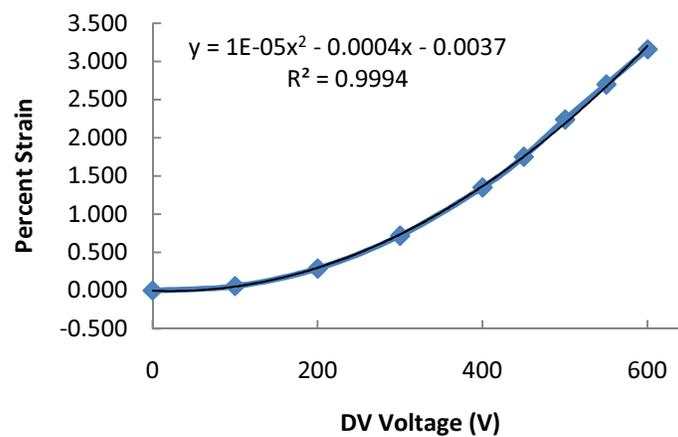
**Figure 4-2: Actuator Strain versus Voltage from Microscopic Camera**
