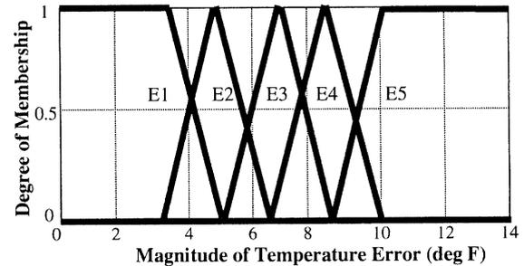
Fig. 3. Membership functions for temperature error.
