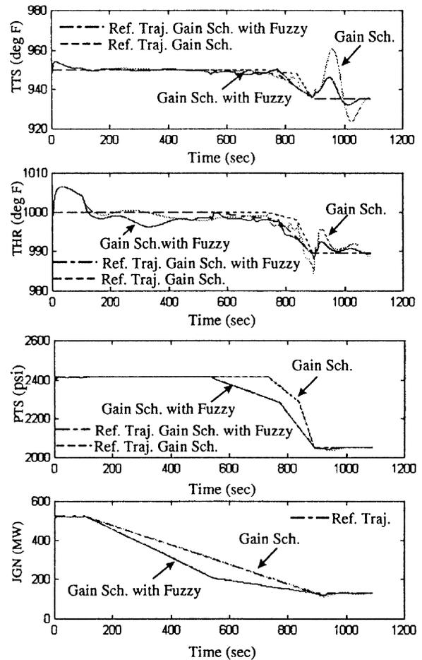
Fig. 10. Ramp down performance of the perturbed plant model.
