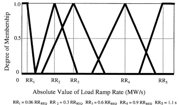
Fig. 4. Membership function for load ramp rate.
