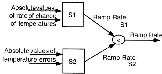
Fig. 5. Parallel processing of the fuzzy control algorithm.
