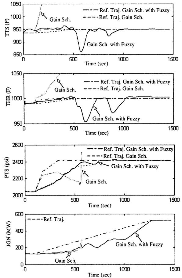
Fig. 12. Ramp up performance of the perturbed plant model.
