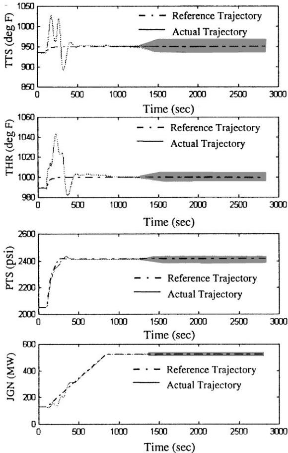
Fig. 7. Ramp-up performance of a single controller in the nominal plant model.
