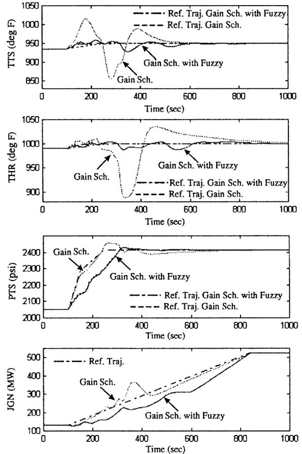
Fig. 8. Ramp-up performance of gain-scheduled controllers in the nominal plant model.
