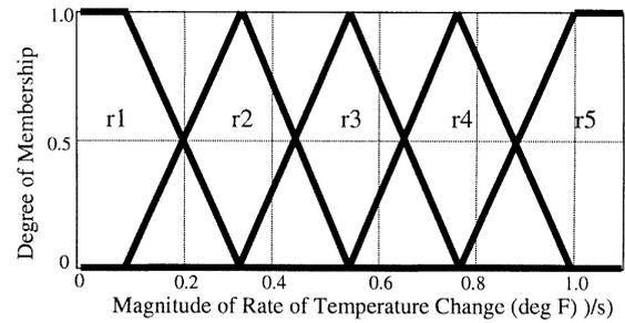
Fig. 2. Membership functions for temperature rate of change.
