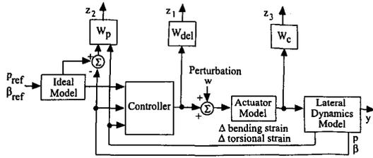
Fig. 4. Generalized plant model for lateral controller design.
