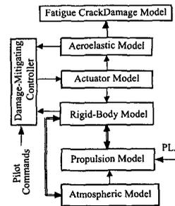
Fig. 3. DMC system schematic.
