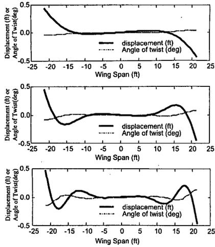
Fig. 2. First three antisymmetric mode shapes.
