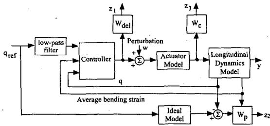
Fig. 5. Generalized plant model for longitudinal controller design.
