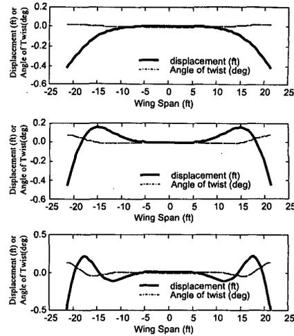
Fig. 1. First three symmetric mode shapes.
