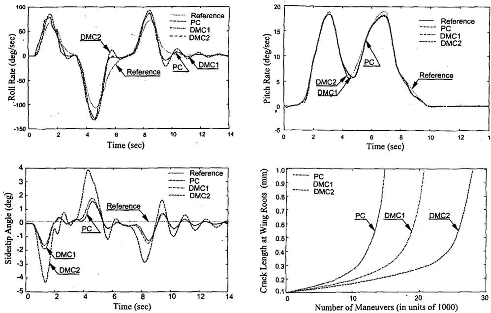
Fig. 6. Aircraft performance and damage under turn reversal maneuver.
