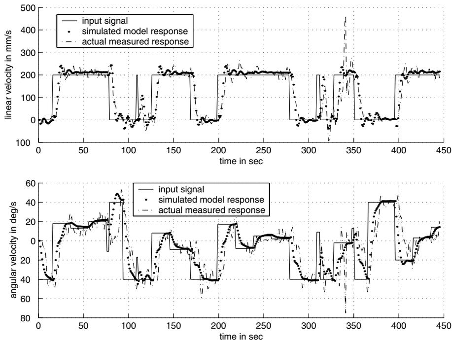
Fig. 3. System identification of the mobile robot.
