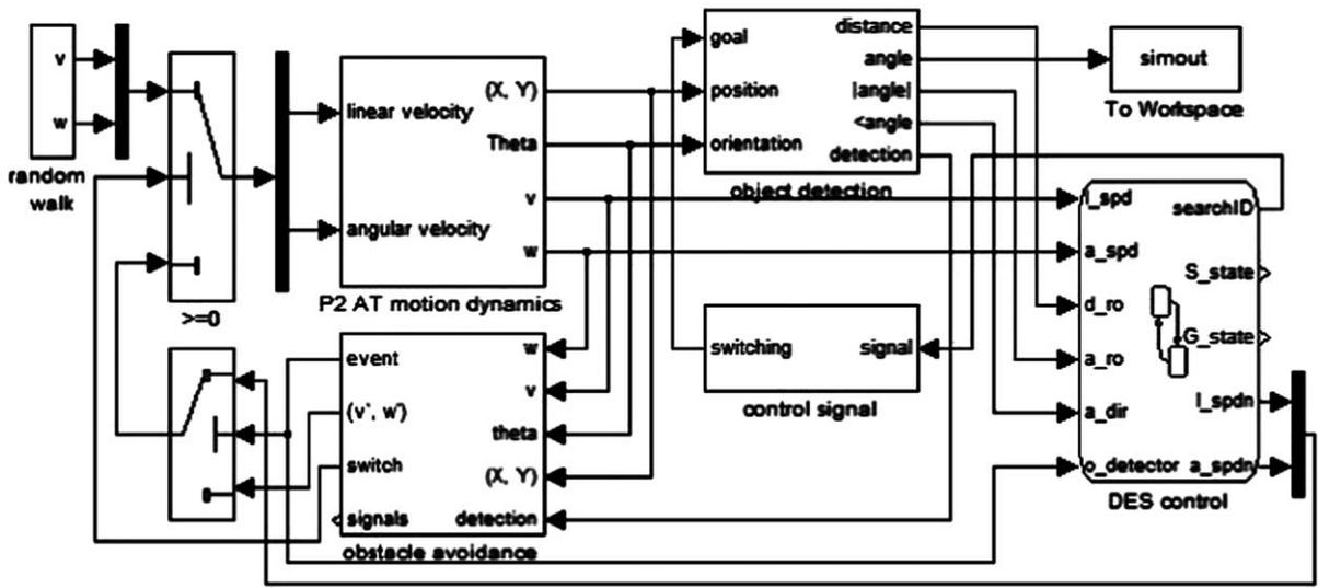
Fig. 2. Matlab robot simulation block diagram.
