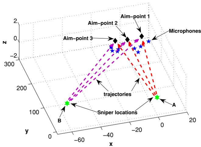
**Figure 3.** A data collection scenario with eight microphones and two rifle locations.
