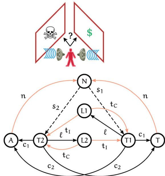
Figure 9. Top: Illustration of the physical scenario, Bottom: Underlying plant model with seven states and eight alphabet symbols: unobservable transitions are denoted by dashed arrows ( - - → ); uncontrollable but observable transitions are shown dimmed ( → ).
