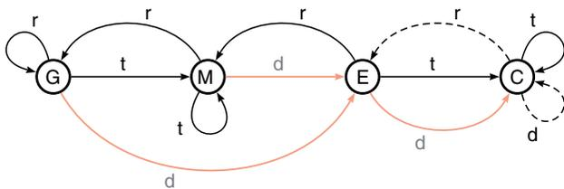
Figure 6. Underlying plant model with four states  $Q = \{G, M, E, C\}$  and alphabet  $\Sigma = \{t, r, d\}$ : unobservable transitions are denoted by dashed arrows ( $- - \rightarrow$ ); uncontrollable but observable transitions are shown dimmed ( $\leftarrow$ ).
