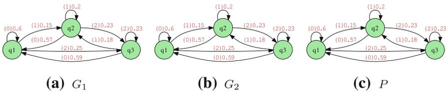
Fig. 6 PFSA representing different motions of robots
