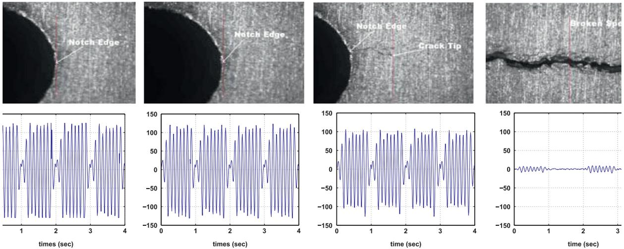
**Fig. 10.** Optical microscope images and ultrasonic time series of surface crack evolution in a 7075-T6 aluminum alloy test specimen. (a) Nominal: 1 kcycles, (b) internal damage: 23 kcycles, (c) surface crack: 34 kcycles, (d) full crack: 47 kcycles.
