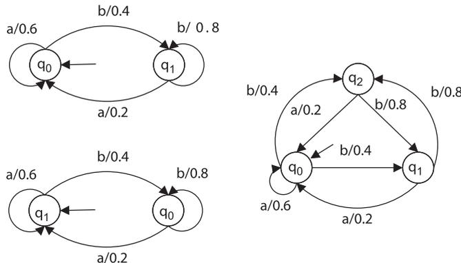
Fig. 2. Different PFSA realizations of the same probability measure.
