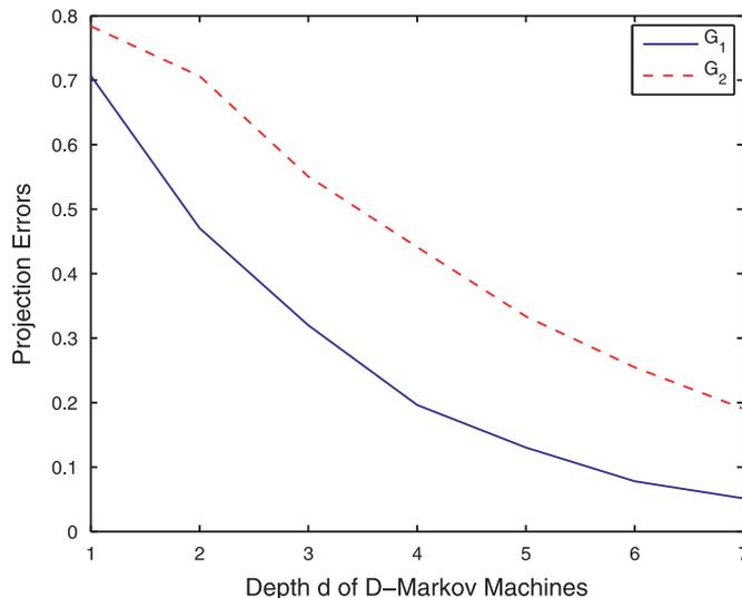
Fig. 7. Projection errors of  $G_1$  and  $G_2$  on  $D$ -Markov subspaces.
