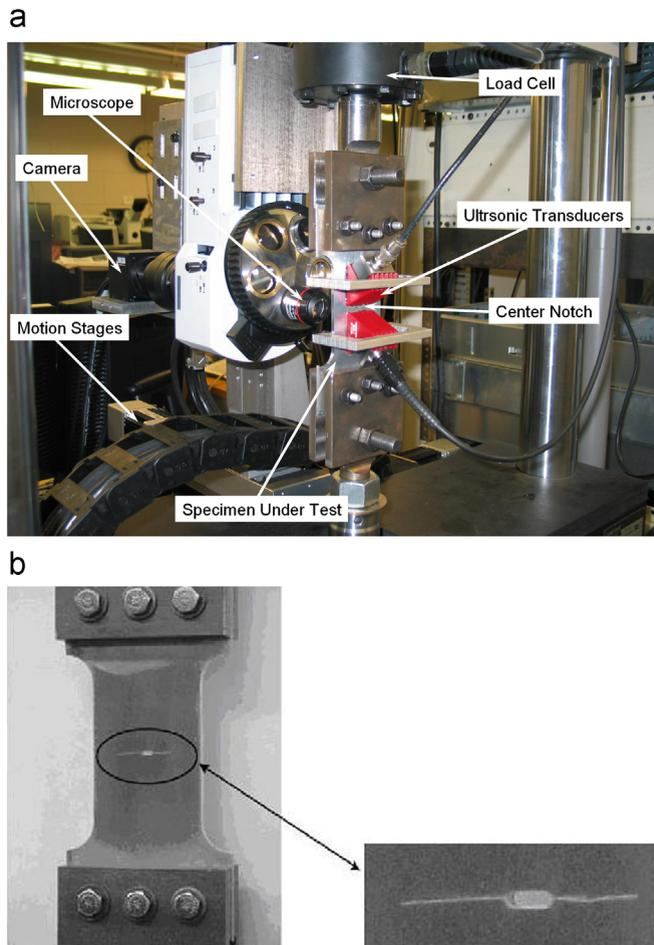
Fig. 9. Computer-instrumented apparatus and a 7075-T6 aluminum alloy specimen. (a) Experimental apparatus, (b) damaged specimen.
