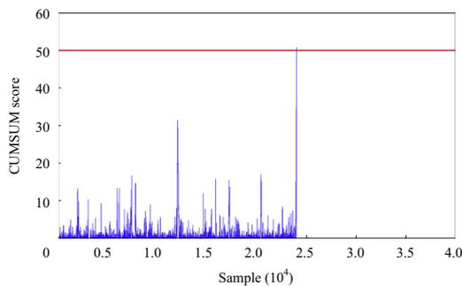
Fig. 9. CUSUM score generated by the variance change detection algorithm on the filtered acoustic signal and the corresponding threshold.
