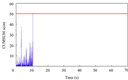
**Fig. 11.** CUSUM score generated by the variance change detection algorithm on the filtered acoustic signal and the corresponding threshold. (After a change in interface is detected, the algorithm restarts.)
