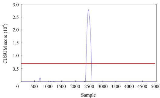
Fig. 7. CUMSU score generated by the mean change detection algorithm on the feed pressure signal and the corresponding threshold.
