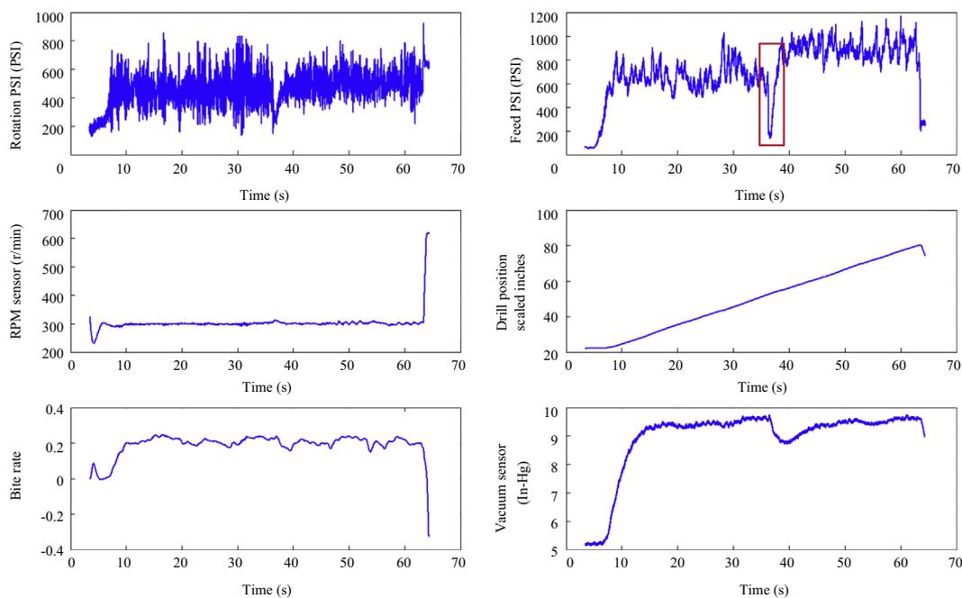
Fig. 3. Typical sensory data collected by the measurement while drilling system of J. H. Fletcher (The measurements correspond to drilling into a stack of two concrete blocks with a void at the intersection of the two concrete block. During the void, the feed pressure signal drops in response to the control unit which regulates the penetration rate).
