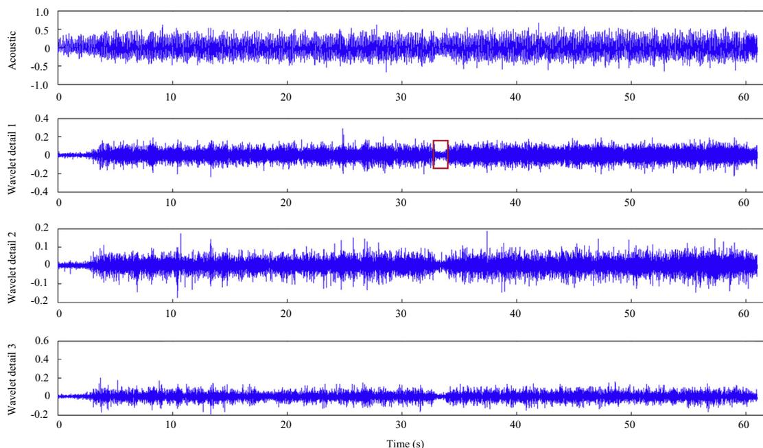
Fig. 4. Acoustic signal (top) and its detailed signals at different levels obtained using 3-level wavelet decomposition with the Daubechies wavelet db3.
