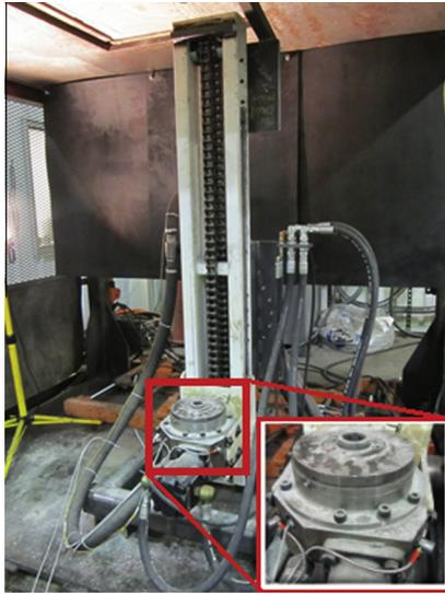
Fig. 2. J. H. Fletcher drill unit equipped with the acoustic and vibration sensors.
