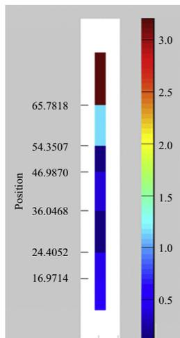
**Fig. 12.** Color-coded variance of each segment relative to the position of the drill bit. (Each segment is identified using the variance change detection algorithm on the filtered acoustic signal.)
