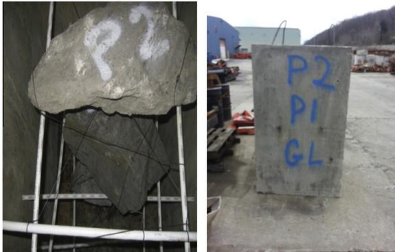
Fig. 6. Rock samples embedded in a concrete to study the correlation of the drilling parameter with respect to the different rock types.
