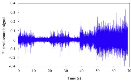
**Fig. 10.** Filtered acoustic signal when drilling into the sandwich of the rocks consisting. (The drill bit reaches concrete->soft rock->concrete->soft rock->concrete->hard rock consecutively.)
