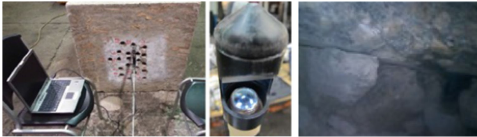
Fig. 9 The screen shot of the view from bore-scoping. (Reproduced with permission from Bahrampour et al. 2014, 2015)
