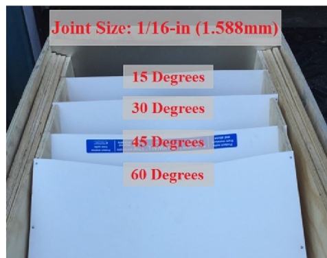
b Simulate inclined joints with Teflon material
