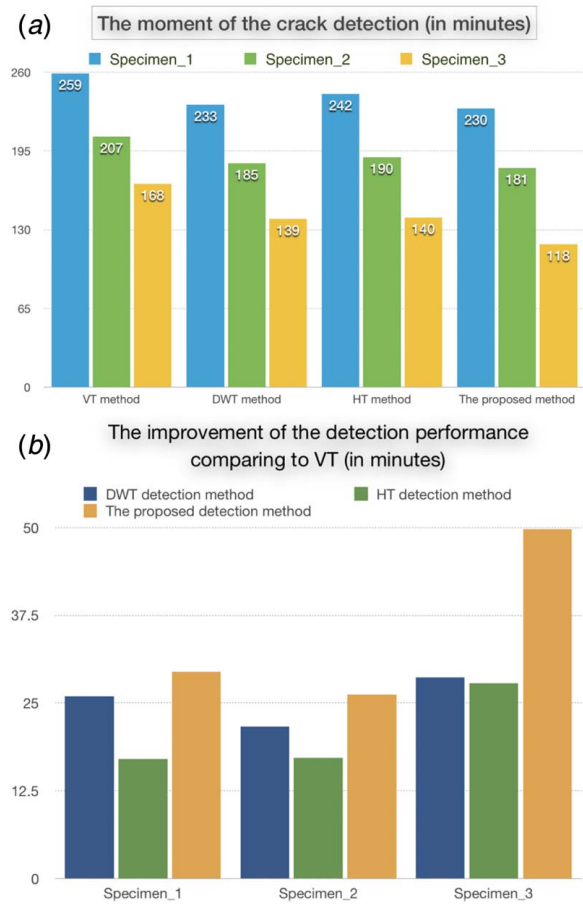
Fig. 27 Comparison study for the moment of the crack detection methods and the improvement of detection performance: (a) instants (min) of crack detection by four methods and (b) reduction in detection time of DWT, HT, and the proposed method as compared to VT
