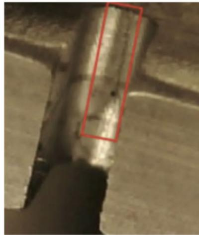
**(b)** Typical visual inspection (VI) image of a crack onset.
