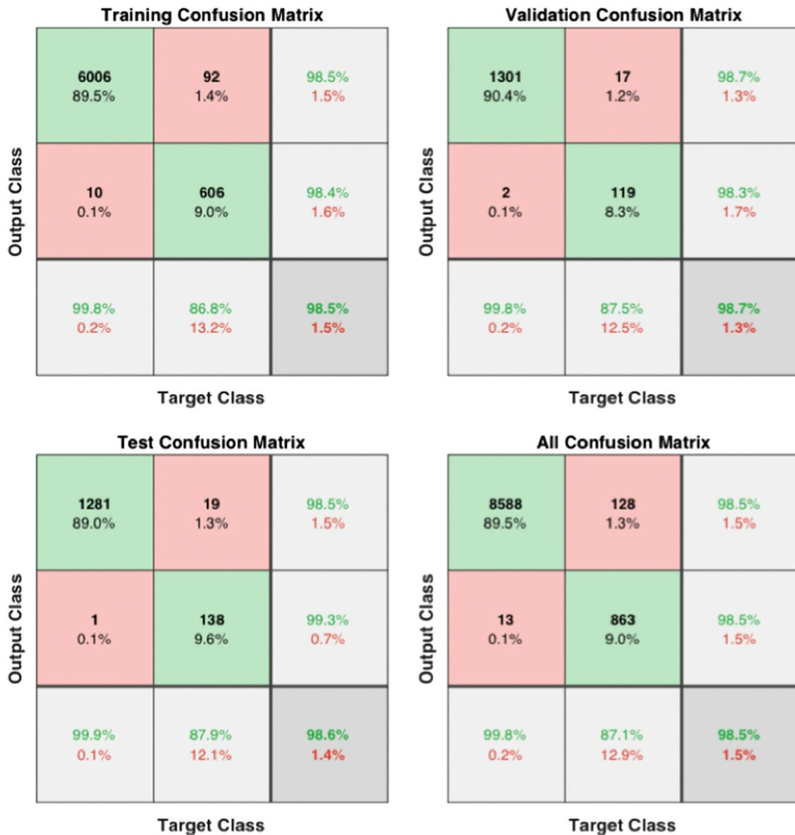
**Fig. 25** Confusion matrices of a typical signals-energy model. In all four subplots, the three regions on each of the abscissa (from left to right) and the ordinate (from top to bottom) indicate the results of undamaged class, damaged class, and overall performance, respectively
