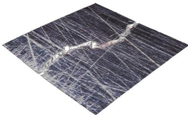
FIGURE 4 Typical 3D surface topography of damaged specimen [Colour figure can be viewed at [wileyonlinelibrary.com](http://wileyonlinelibrary.com)]
