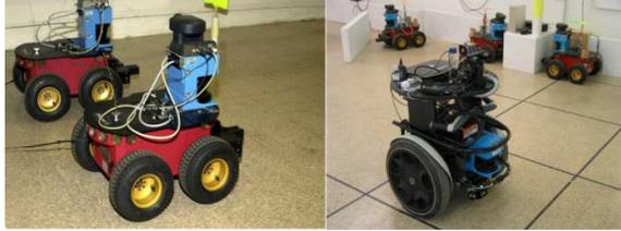
FIGURE 1.5: The Robot Hardware: Pioneer 2AT (Left) and Segway RMP (Right)
