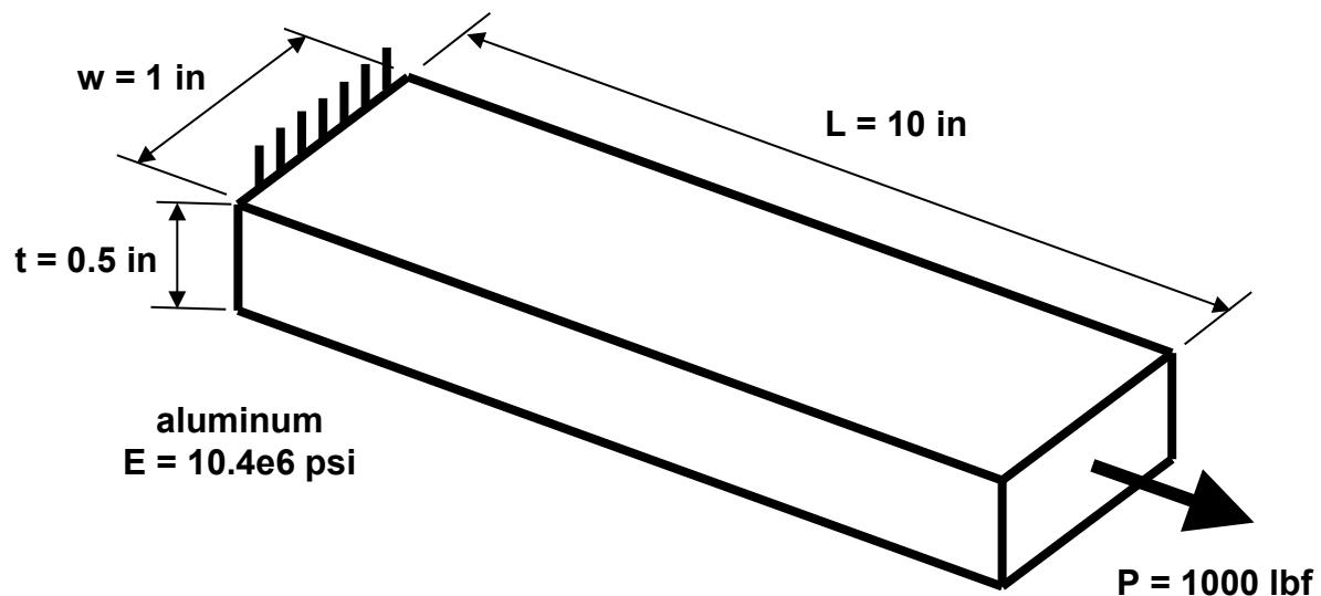
$$\delta = \frac{P L}{A E} = \frac{P L}{t w E} = \frac{(1000 \text{ lbf})(10 \text{ in})}{(0.5 \text{ in})(1 \text{ in})} \left( \frac{\text{in}^2}{10.4 \times 10^6 \text{ lbf}} \right) = 0.001923 \text{ in} = 1.923 \text{ mil}$$
