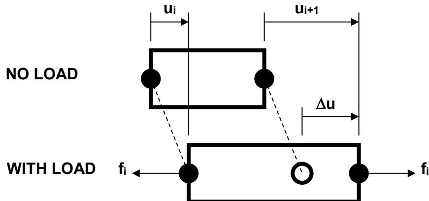
$$\Delta u = \frac{f_i l_i}{A_i E_i} = \frac{f_i l_i}{t_i w_i E_i} \quad f_i = \frac{t_i w_i E_i}{l_i} (\Delta u) = k_i (\Delta u) = k_i (u_{i+1} - u_i) \quad k_i = \frac{t_i w_i E_i}{l_i}$$
