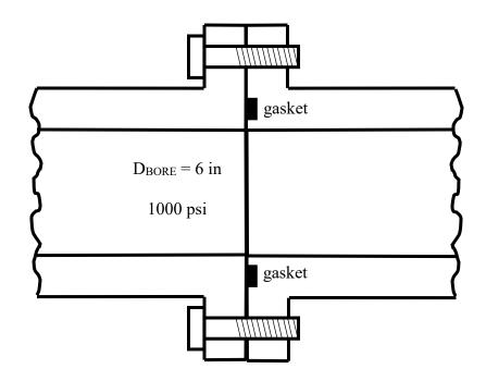
6 inch ID pipe with flanges 1040 cold rolled steel 1000 psi pressure 12 bolts around flange 1/2-20 UNF Grade 8 threaded into flange application factor of safety  $N_{AFS} = 2$  to prevent blow-by
