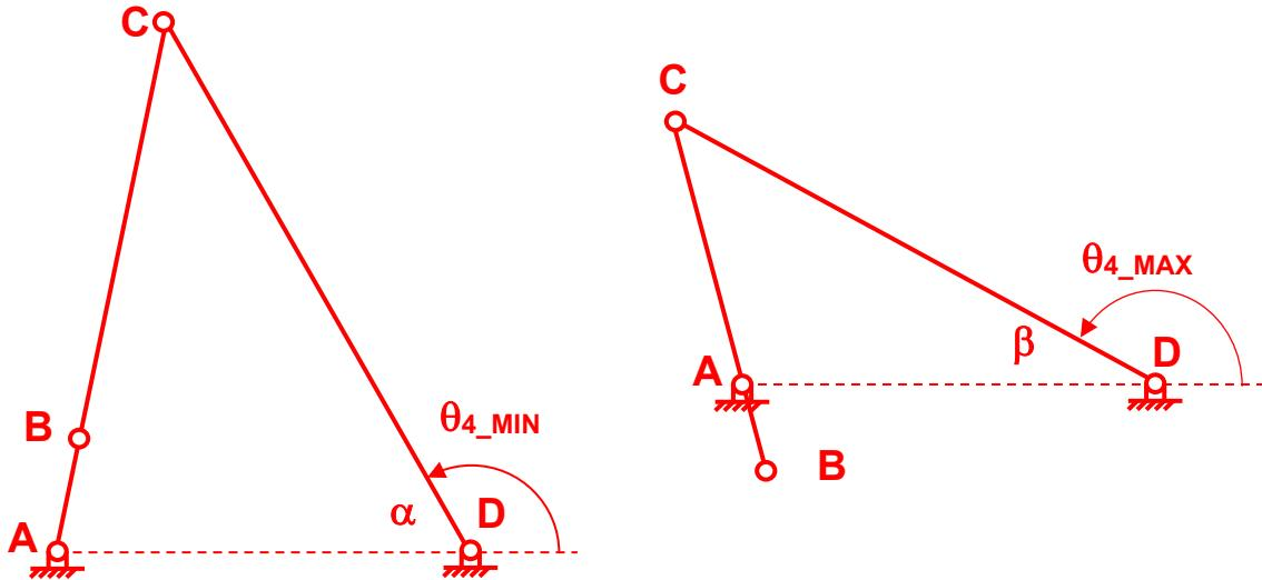
$$(BC + AB)^2 = AD^2 + CD^2 - 2(AD)(CD)\cos\alpha \quad \alpha = 66.4218^\circ \quad \theta_{4\_MIN} = 113.5782^\circ$$
