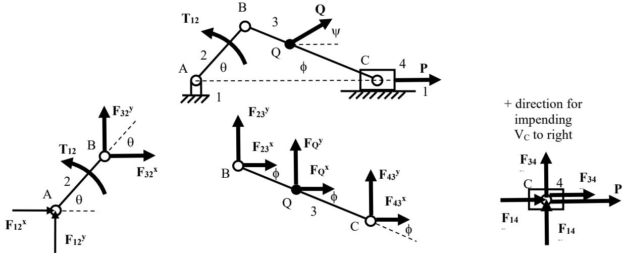
$$\Sigma F \text{ on 2 right} + F_{12}^x + F_{32}^x = 0$$
