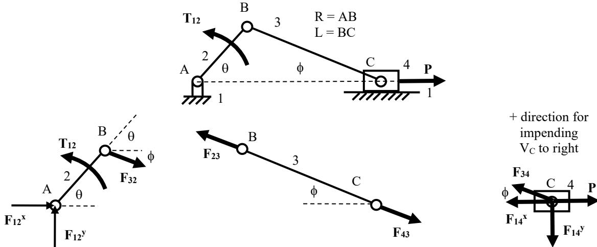
$$\Sigma F \text{ on 4 right } + P - F_{14}^x \text{ sign}(V_C) - F_{34} \cos\phi = 0$$
