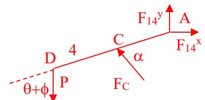
$$\sum M \text{ on } 4 \text{ about } A \text{ CCW} + \\ -(F_c \sin \alpha) AC + (P \sin(\theta + \phi)) AD = 0 \\ F_c = 2261.9 \text{ lbf}$$
