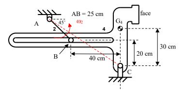
$$\begin{aligned} m_4 &= 2.3 \text{ kg} \\ J_{G4} &= 30 \text{ N.cm.sec}^2 \\ \omega_2 &= 50 \text{ rpm CCW constant} \\ \omega_4 &= 2.32 \text{ rad/sec CW} \\ \alpha_4 &= 20.13 \text{ rad/sec}^2 \text{ CW} \end{aligned}$$
