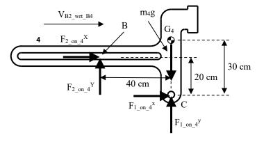
$$+ F_{2_{on}} A^{X} + F_{1_{on}} A^{X} = m_{4} A_{G4}^{X}$$
