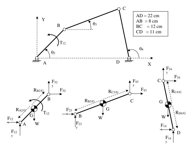
Weights are true external forces caused by gravity. d'Alembert inertial forces and moments may be treated as if they were external forces/moments acting on the links.
