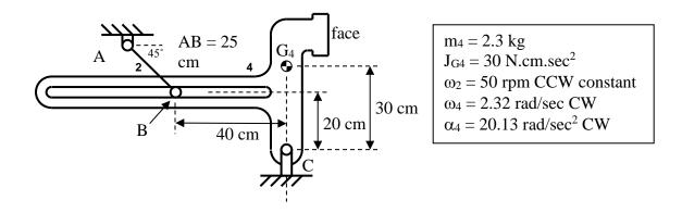
Determine the magnitude and direction of motor torque  $T_{1\_on\_2}$  on crank 2 required to cause this motion at this position.
