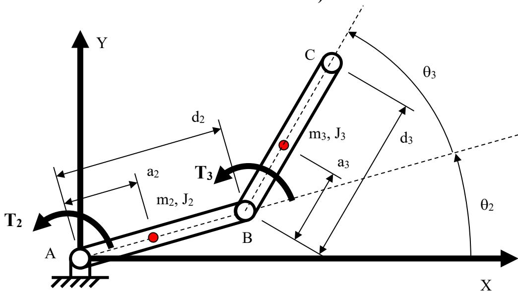
Two solid rigid bars with revolute joints A and B
