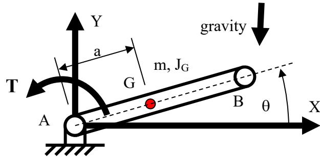
$$q = \theta \quad \dot{q} = \dot{\theta} \quad \ddot{q} = \ddot{\theta} \quad Q = T$$
