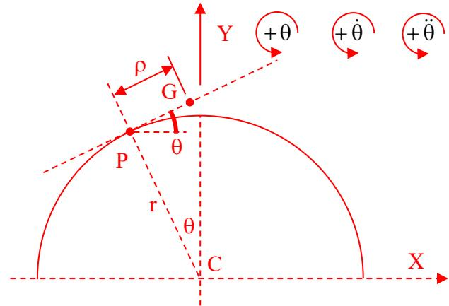
$$\frac{d}{dt} \left( \frac{\partial L}{\partial \dot{\theta}} \right) - \frac{\partial L}{\partial \theta} = 0 \quad 2m r^2 \theta \dot{\theta}^2 + m r^2 \theta^2 \ddot{\theta} + J \ddot{\theta} - (m r^2 \theta \dot{\theta}^2 - m g r \theta \cos \theta) = 0$$
