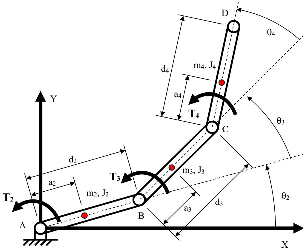
Three solid rigid bars with revolute joints A, B and C
