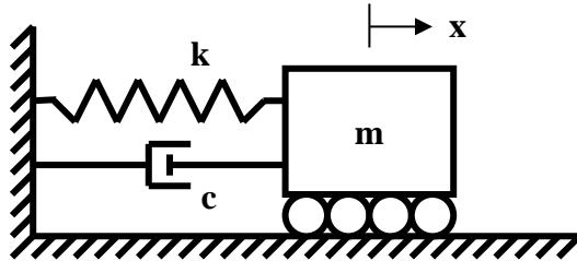
$$m\ddot{x} + c\dot{x} + kx = 0 \quad \ddot{x} = -\frac{k}{m}x - \frac{c}{m}\dot{x}$$
