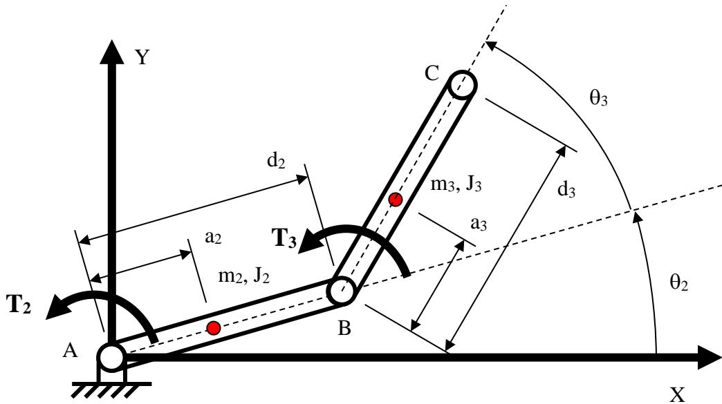
Two solid rigid bars with revolute joints A and B
