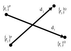
$\left\{r_{i}\right\}^{P}+d_{i}\left(\left\{r_{i}\right\}^{Q}-\left\{r_{i}\right\}^{P}\right)=\left\{r_{j}\right\}^{P}+d_{j}\left(\left\{r_{j}\right\}^{Q}-\left\{r_{j}\right\}^{P}\right) \qquad \text{ intersect } if \quad 0\leq d_{i}\leq 1 \quad \text{and} \quad 0\leq d_{j}\leq 1$
