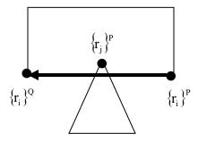
given candidate vertex  $\{r_j\}_t^p$  on body j that collides with body i at time t given candidate edge  $\{r_i\}_t^Q - \{r_i\}_t^p$  on body i that has two edge intersections with body j at time t must know position and velocity for all three points at time t-h (time step h)
