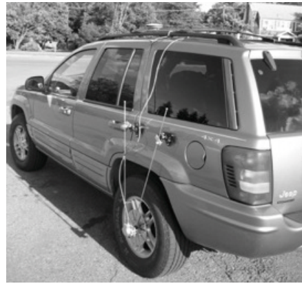
Fig. 2. Side view of the test vehicle shown with the wheel odometer and GPS antenna.
