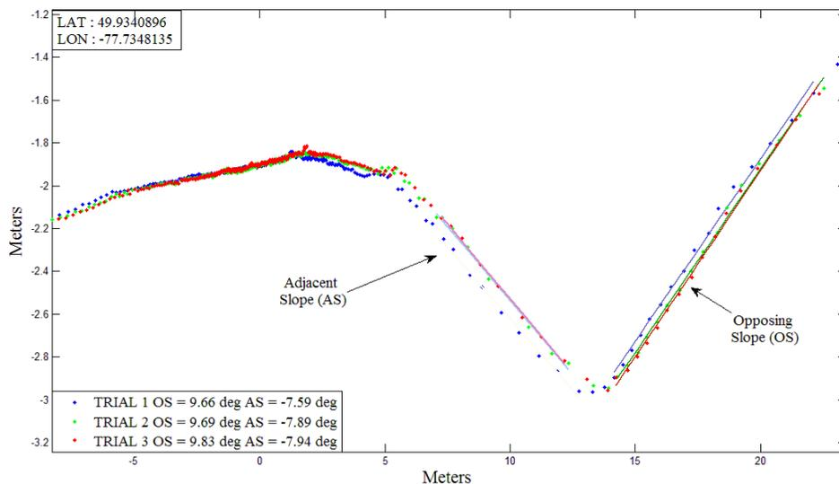
**FIGURE 8: LIDAR scans obtained in three different runs at a known GPS location**
