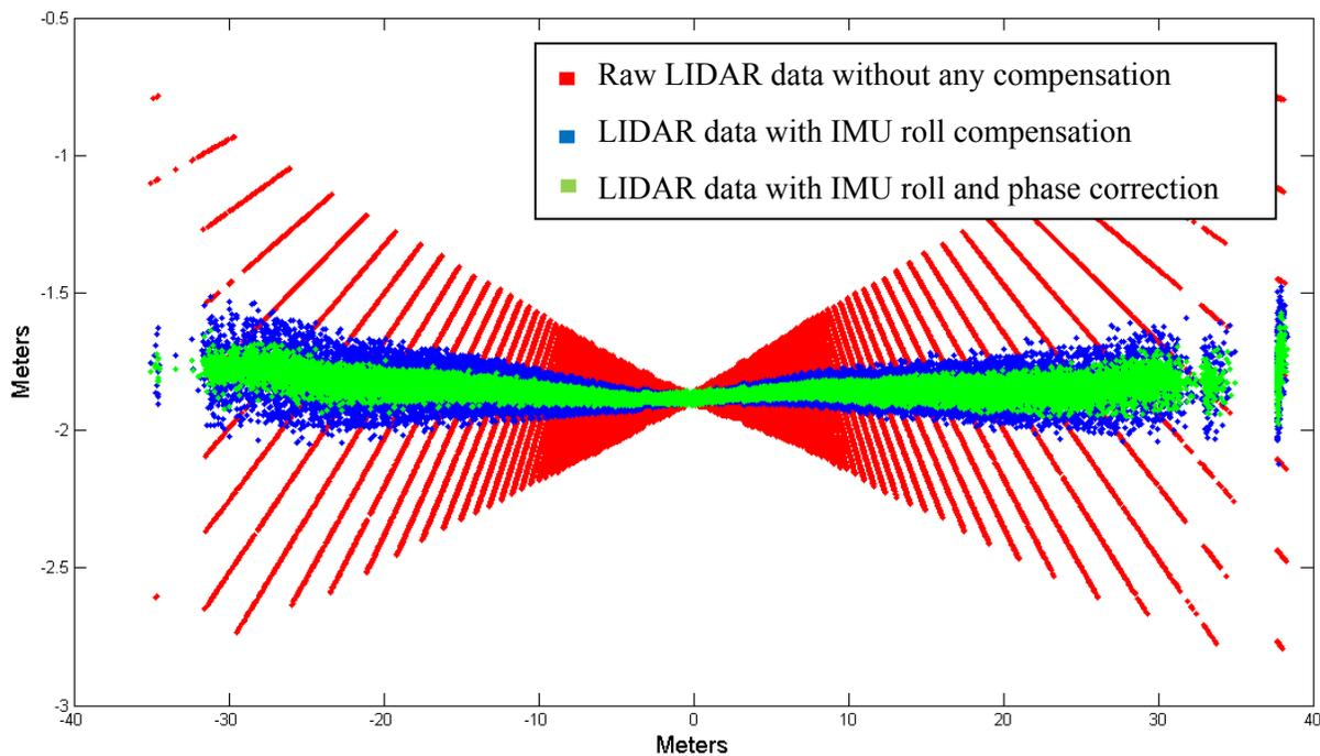
**FIGURE 6: The figure shows the horizontal surface underneath the laser, under different levels of correction for the vehicle roll.**
