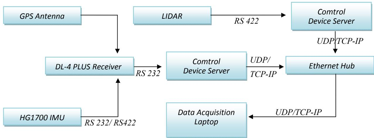
**FIGURE 3: Data Routing Architecture**
