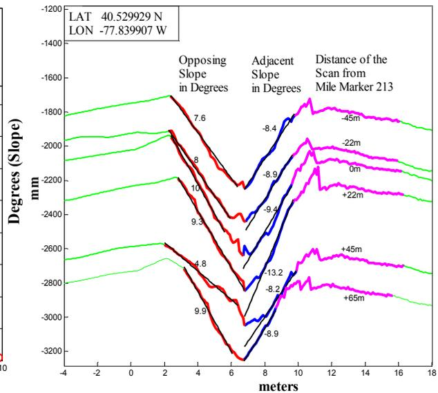
**FIGURE 9b:** The plot illustrates the variation of the median profile along a distance of +/- 50 meters around mile
