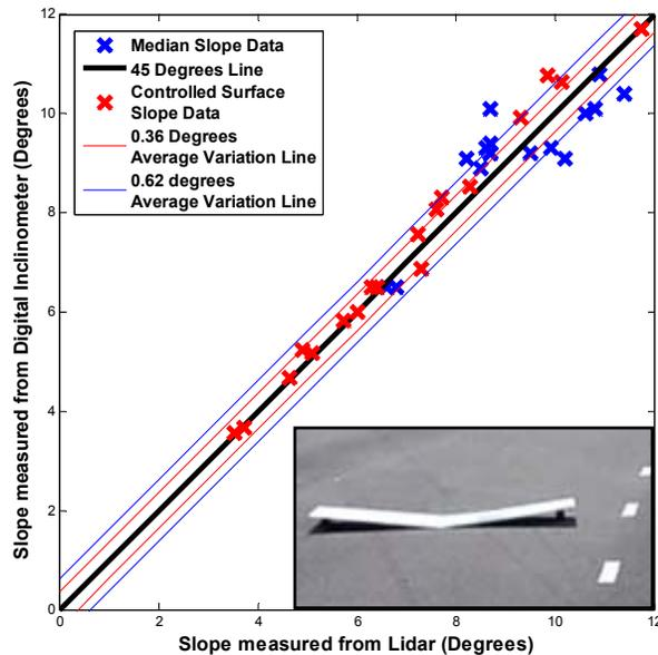
**FIGURE 7a: Comparison of LIDAR slope measurements to manual slope measurements. The control surface used for the measurements is shown in the picture to the corner.**
