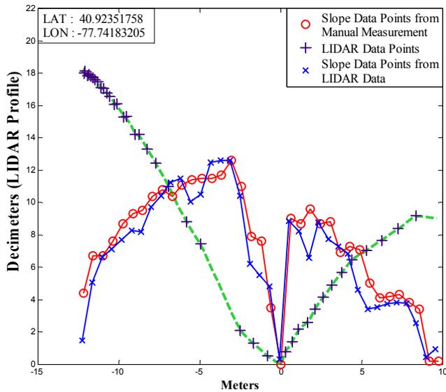
**FIGURE 9a:** The variation of the slope along the profile of a median cross section measured manually and with LIDAR
