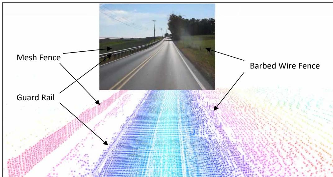
**FIGURE 10:** 3-D visualization of LIDAR point cloud, taken at Foxhill Road westbound, State College, PA.
