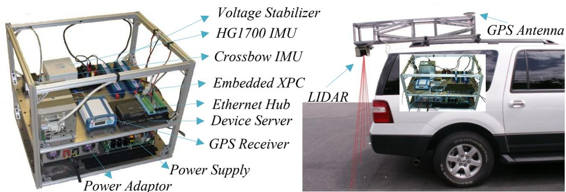
**FIGURE 1: Data acquisition system**
