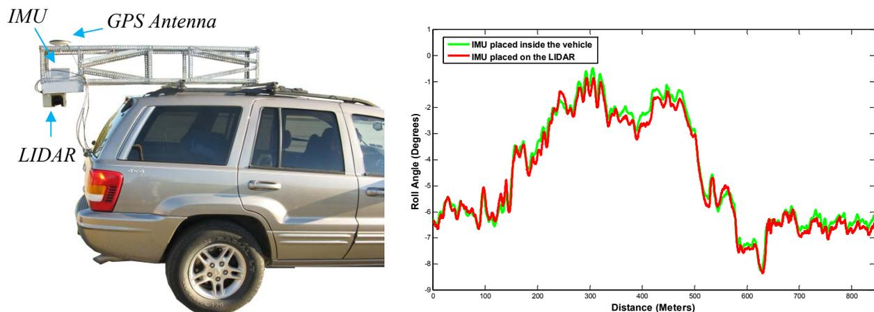
**FIGURE 2:** The figure shows the roll measured under two different conditions in which the IMU is placed inside the vehicle (Figure 1) and on the LIDAR (as seen in the above picture).
