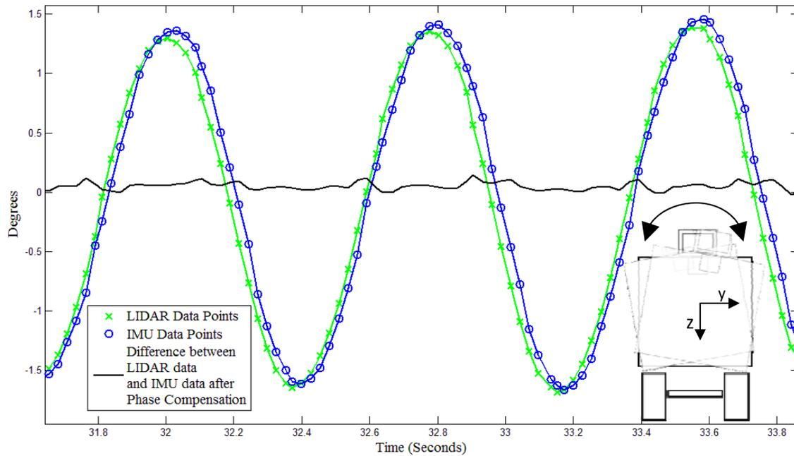
**FIGURE 5: The figure illustrates the ability of the IMU data to compensate for the roll experienced by the vehicle.**
