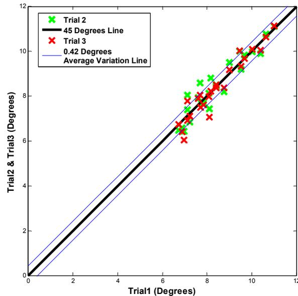
**FIGURE 7b: Repeatability test for LIDAR slope measurement at different known GPS locations**
