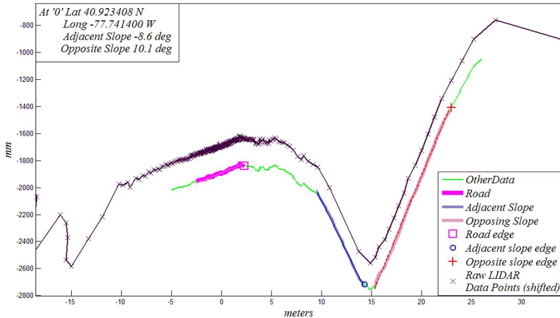
**FIGURE 4: The processed scan data for a typical road cross section showing the Road, the adjacent slope and the opposing slope as identified by the algorithm. (The Raw LIDAR scan data has also been shown and has been shifted up for visibility)**
