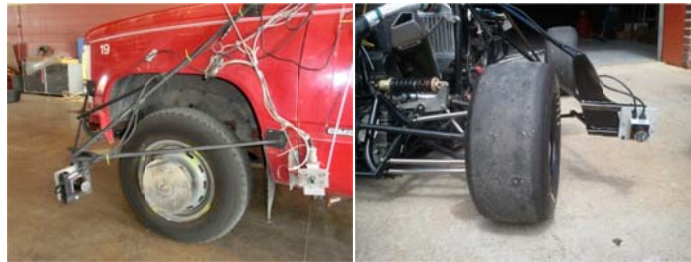
Figure 2: Physical mounting of the LIDAR sensor over the wheel plane for a GMC truck and F SAE vehicle.
