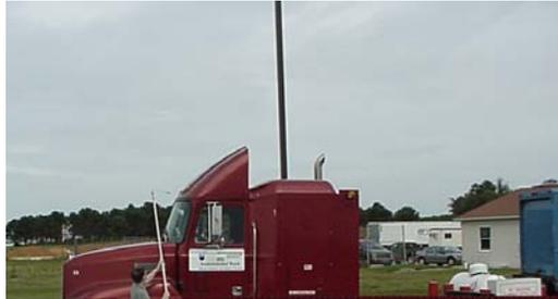
*Figure 3.4: The arm is shown capable of measuring points along the front of the vehicle as well, provided that the stylus is bent to be at a ninety-degree angle to the axis of the link to which it is mounted.*
