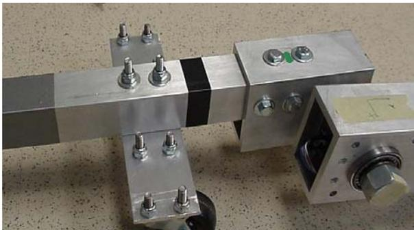
Figure 6.20: Dual castor wheels are mounted to a plate at end of 5<sup>th</sup> link.
