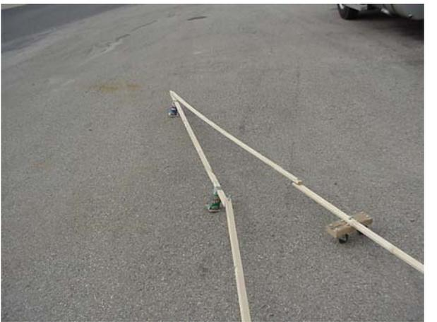
*Figure 3.6: As the end of the arm continued to be moved towards the armature base, the same folded up configuration, shown in Figure 5, appeared again, one joint closer to the base. Once, again, this configuration unfolded itself when continuous force was applied to the end linkage.*
