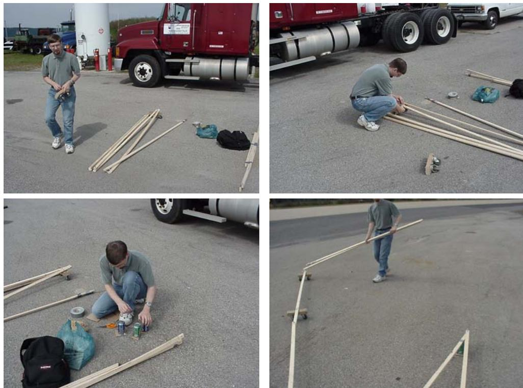
*Figure 3.1: The mockup armature was assembled at the PTI test track. The arm was transported in a folded up state (upper left). Caster wheels were mounted to cross pieces, which were in turn mounted to the arm (upper right). Sodas cans, with cardboard bases, were taped to the bottom of the armature to keep the device level (lower left). The mockup was unfolded by pulling on the two links closest to the stylus (lower right).*
