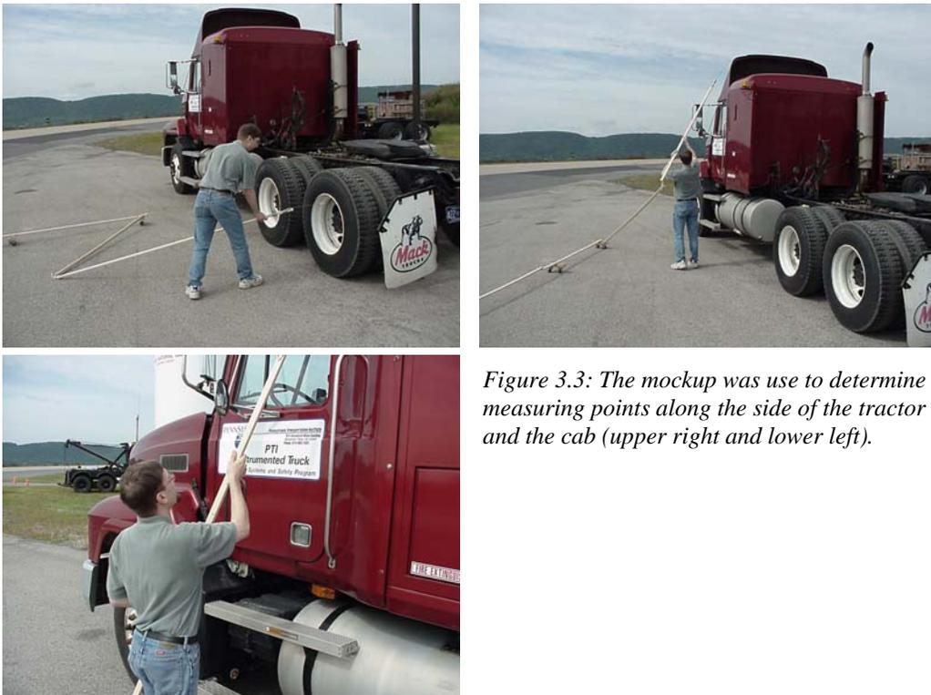
*Figure 3.3: The mockup was use to determine the feasibility of measuring points along the side of the tractor chassis (upper left) and the cab (upper right and lower left).*
