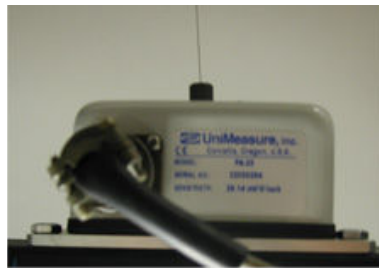
Figure 4.2: String Potentiometer Used for Steering Angle Measurement
