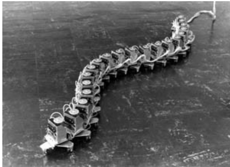
Figure 1.1: The Active Cord Mechanism (ACM III)
