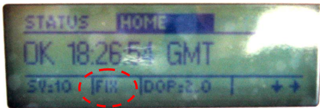
Figure C.3: Receiver with Fixed Position
