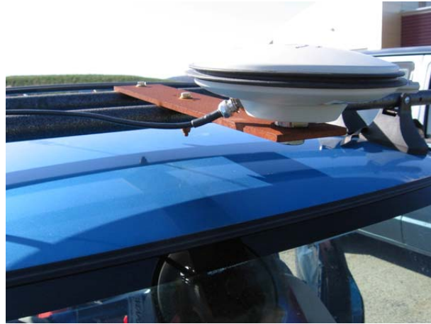
Figure C.5: GPS Antenna Mounting
