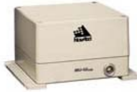
Figure 4.3: Honeywell HG1700 IMU – NovAtel Enclosure
