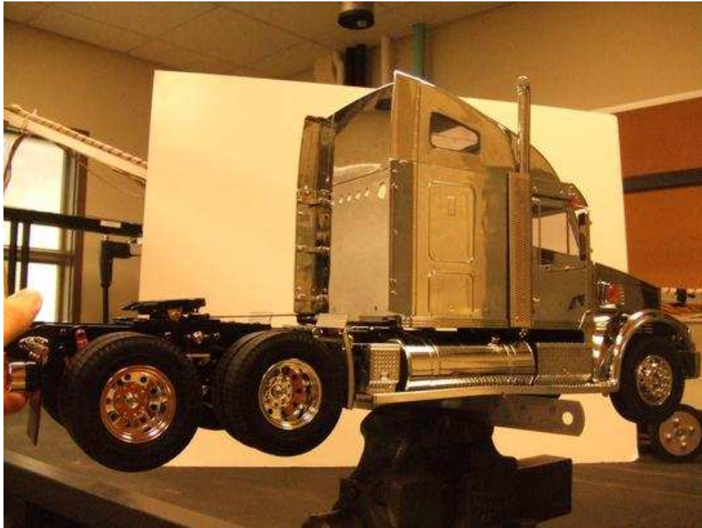
Figure 4.1: Balancing the tractor to locate its center of gravity
