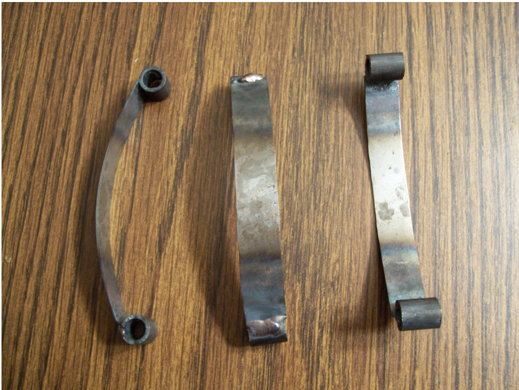
Figure 3.7: This picture shows three finished leaf springs from three different views. All are the same overall length, and they have the same radius of curvature.
