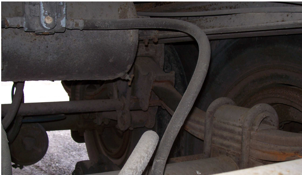
Figure 3.5: Note the two leaf springs on each side of the trailer, one on each axle
