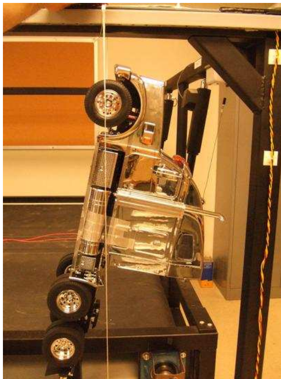
Figure 4.2: Suspending the Model from the front axle to determine the vertical location of center of gravity
