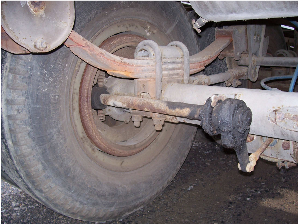
Figure 3.4: A leaf spring attached to the axle on the full size trailer
