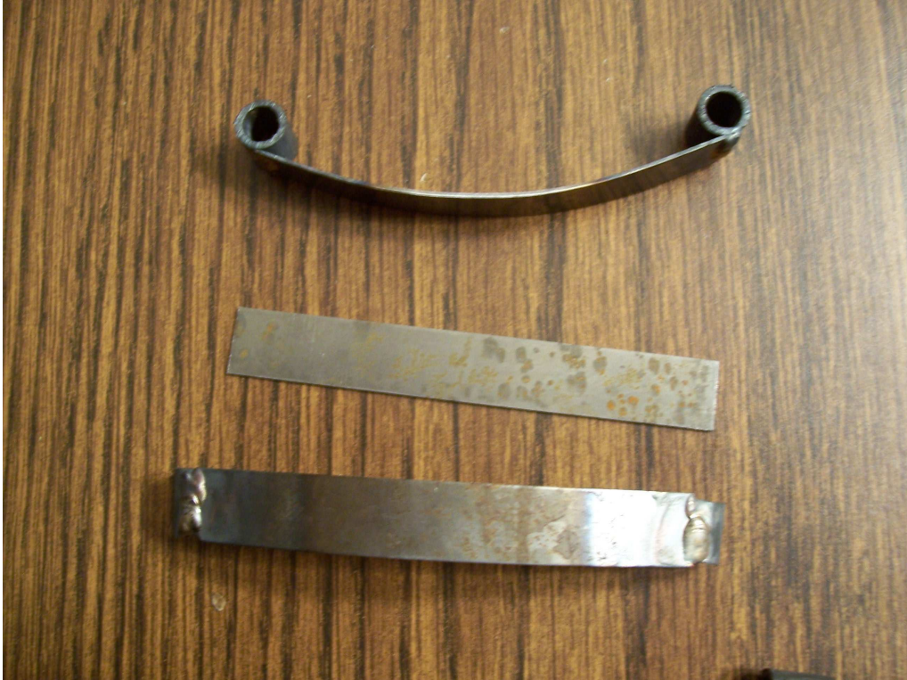
Figure 3.6: This picture shows the original size of the metal strip along with two completed leaf springs. Note that though the strip is bent, the finished springs are longer due to the connectors.
