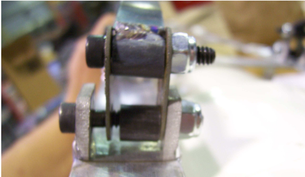
Figure 3.9: This is the rear view of the suspension. The spacer on the bottom bolt keeps the suspension pivots vertical, allowing for a consistent ride height on each spring
