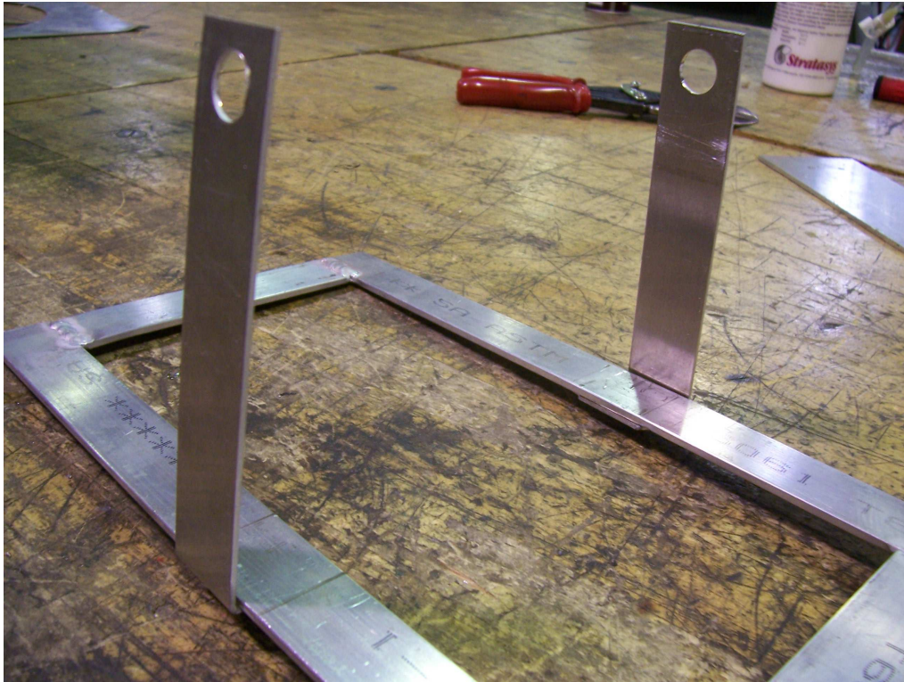
Figure 3.14: The lateral supports bent slightly past 90°, with holes punched to accommodate zip ties
