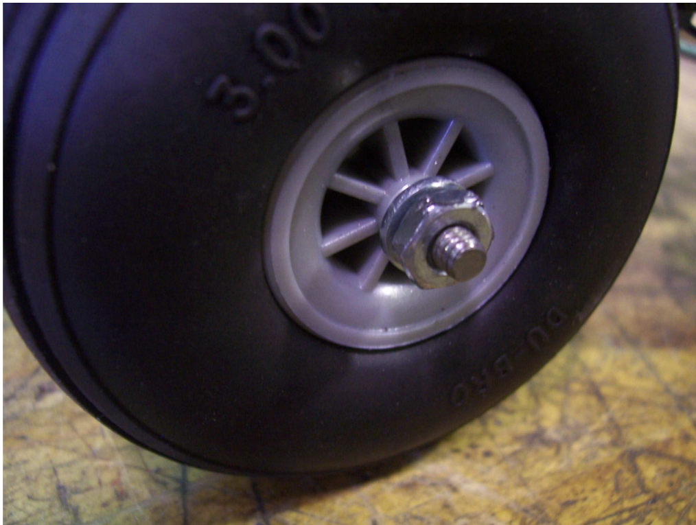
Figure 3.13: A close up of the fastening mechanism on one of the axles.
