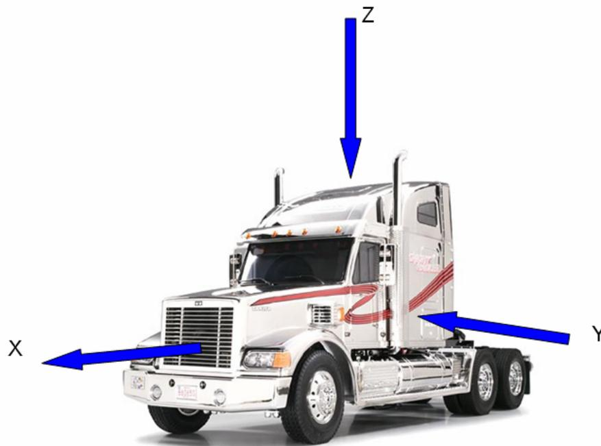
Figure 3-2: Body-fixed coordinate system
