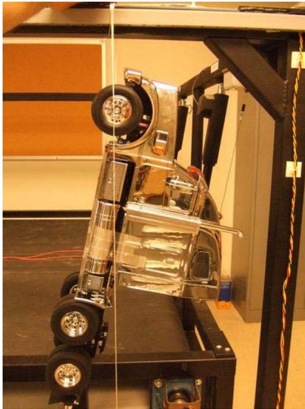
Figure 5-3: Estimating the mass moment of Inertia
