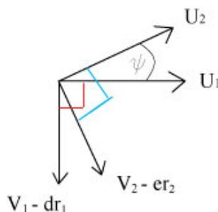
Figure 2-4: Velocities at the fifth wheel for both the tractor and trailer.
