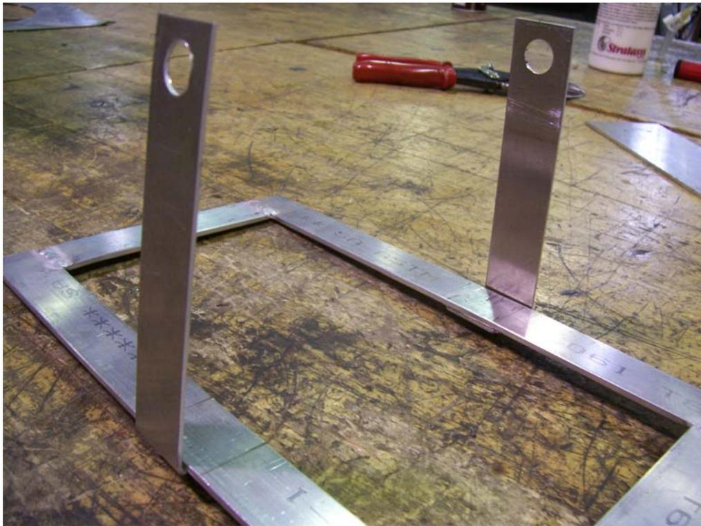
Figure 4-9: L brackets for securing the tank and container.
