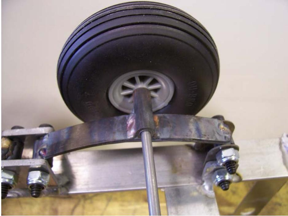
Figure 4-6: The axle running through the sleeve on the front driver side leaf spring
