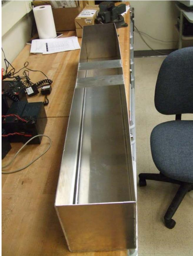
Figure 4-12: The finished container with two braces in the middle to help keep the container from deforming.
