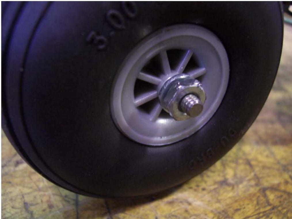
Figure 4-8: The trailer wheel and a washer secured with a nut
