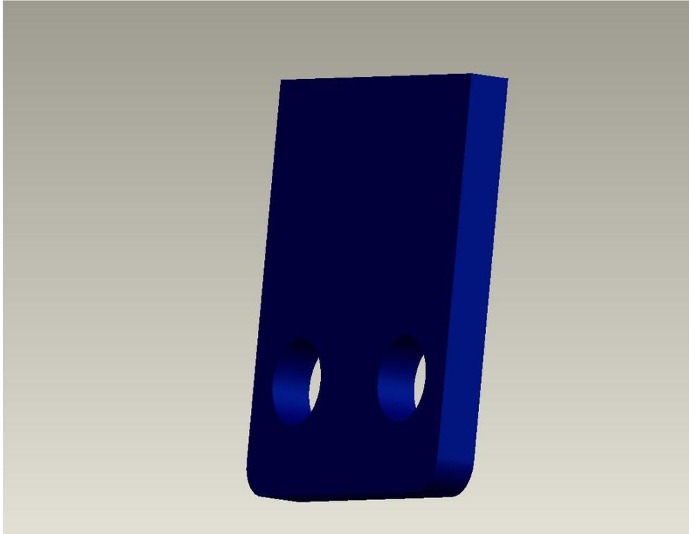
Figure D-2: Pro/E Model of the Center Spring Mounts
