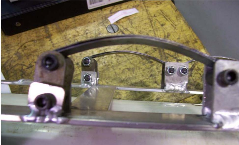
Figure 4-3: Front leaf spring and its connections to the chassis
