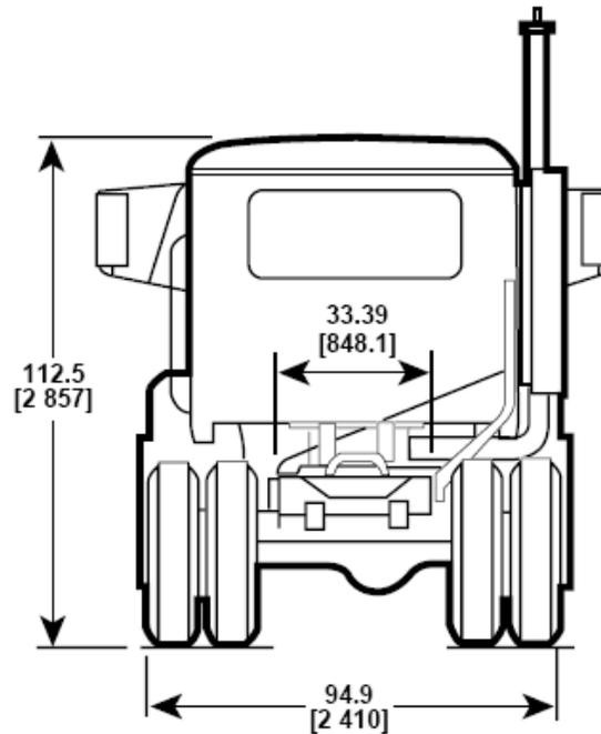
Figure A-1: The parameters from the Mack Truck specifications [1]
