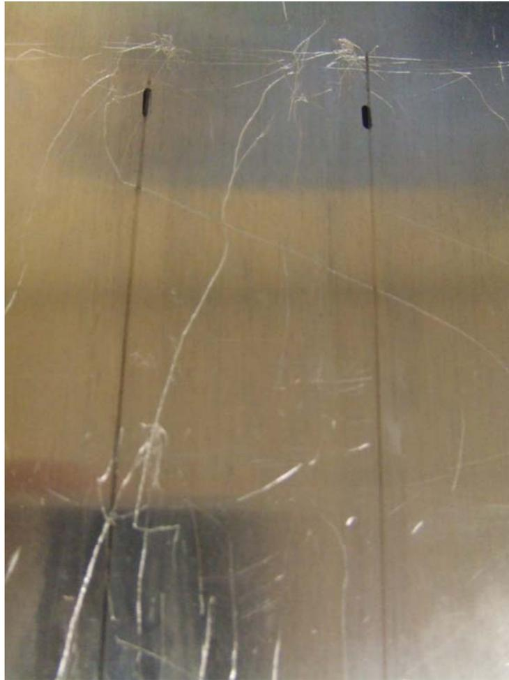
Figure 5-4: Two of the twelve marks placed on the container to ensure the container has not slid relative to the chassis
