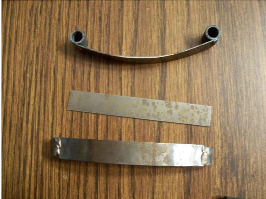
Figure 4-2: Two formed leaf springs on the top and bottom with one unformed strip in the center.
