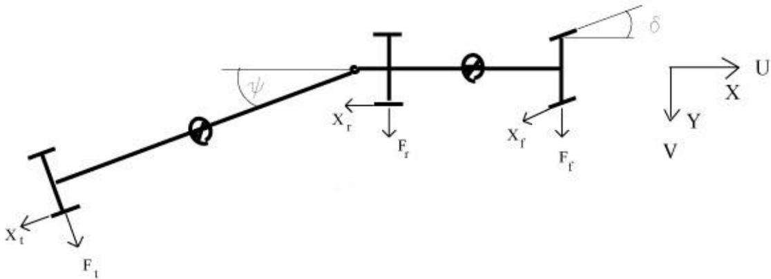
Figure 2-5: Forces acting on the tractor-trailer system
