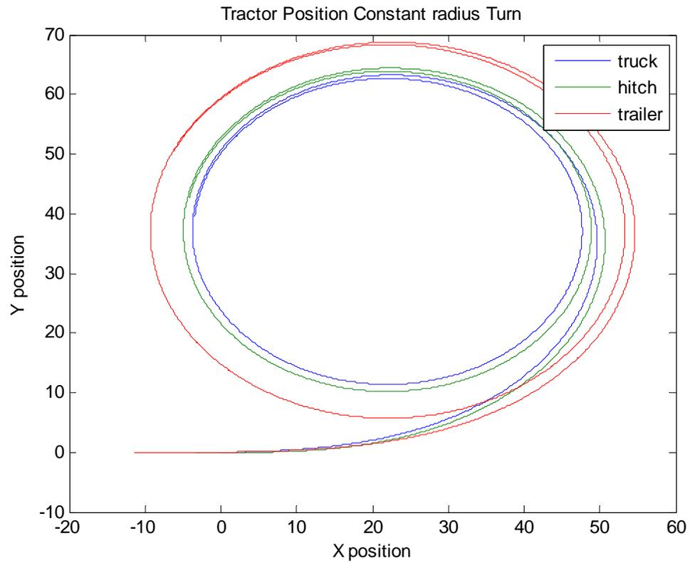
Figure B-4: The simulated response for a constant radius turn at 15 m/s and a constant steering angle of 7 degrees = 0.122 radians
