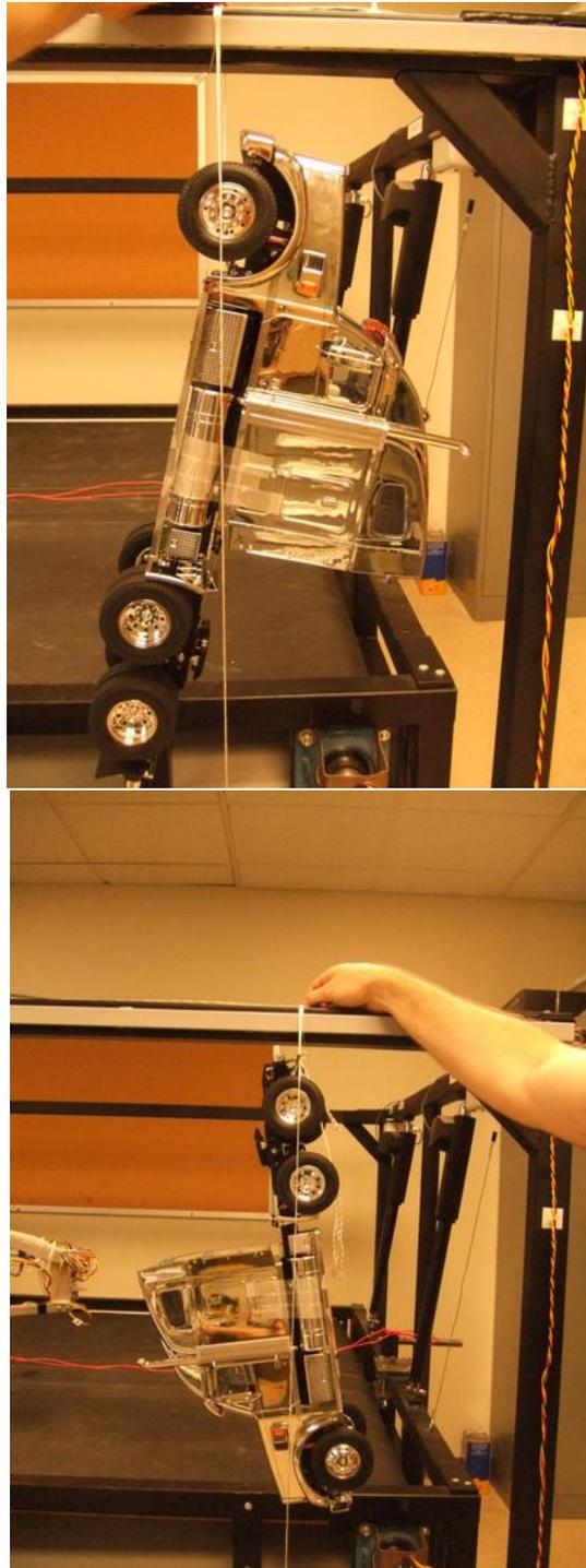
Figure 5-2: Estimating the height of the center of gravity by hanging the scaled vehicle from the front and rear axles.
