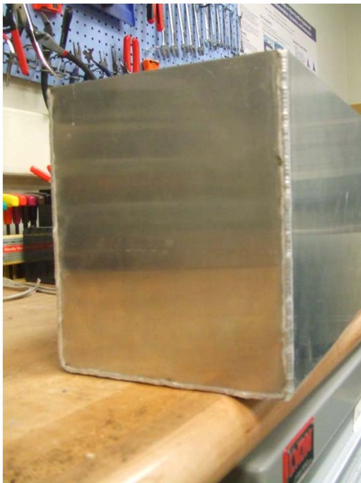
Figure 4-11: One of the end pieces welded inside the “U” shaped container.
