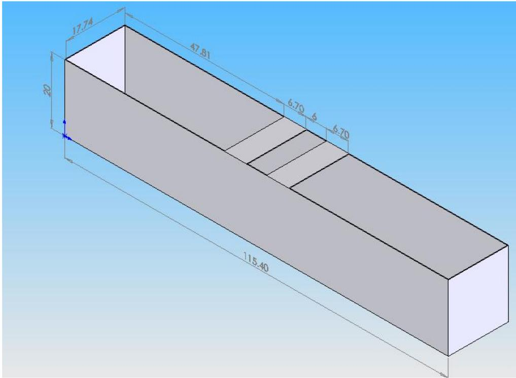
Figure D-5: SolidWorks Model of the container with dimensions in centimeters
