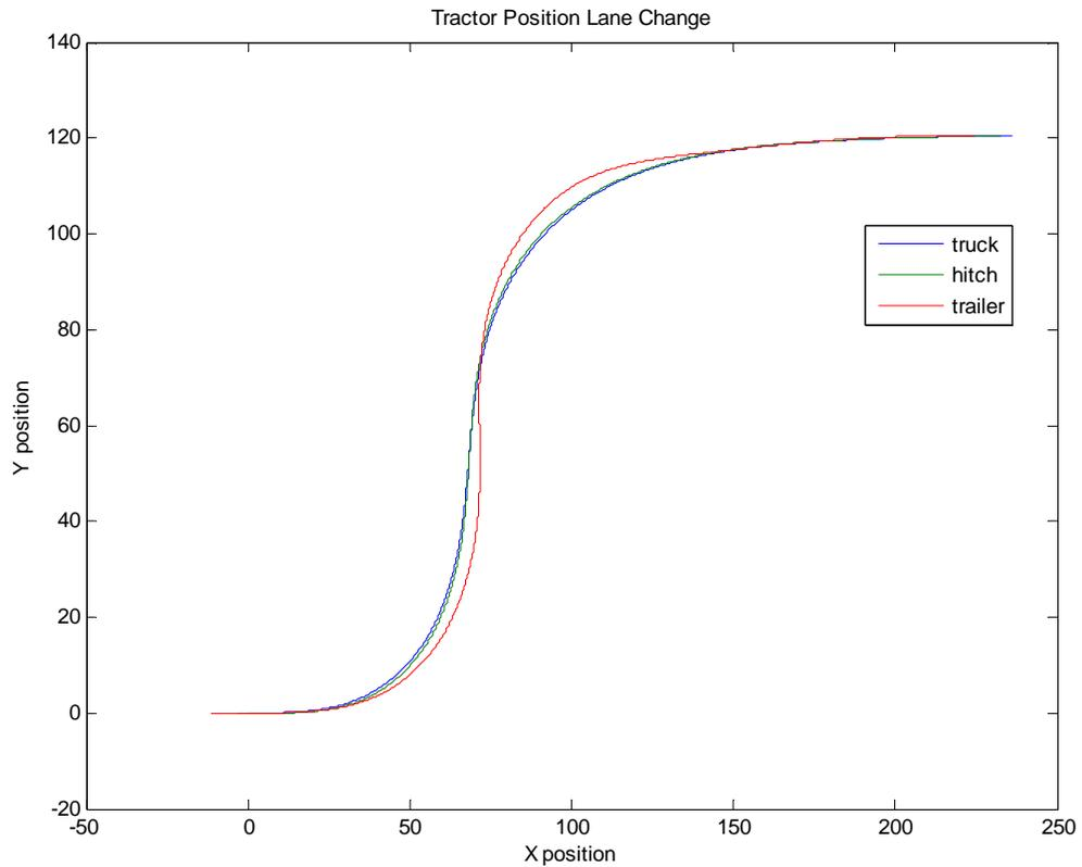
Figure B-3: The simulated response to a lane change maneuver at 25 m/s and a steering angle of 0.5 degrees = 0.0087 radians. Once again the tractor trailer system responds as expected. As the speed of the tractor trailer continues to increase the trailer continues to follow a path closer and closer to that of the truck. However, at excessive speeds as in the graph above, the trailer eventually swings out past the path followed by the truck.
