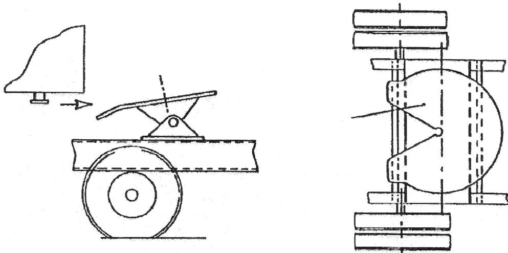
Figure 2-1: The fifth wheel connects the trailer to the tractor, from Road Vehicle Dynamics by J R Ellis[2]
