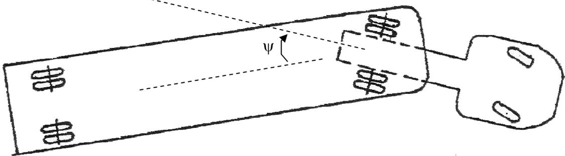
Figure 2-2: A tractor and trailer combination with an articulation angle  $\neq 0$ , from Road Vehicle Dynamics by J R Ellis[2]
