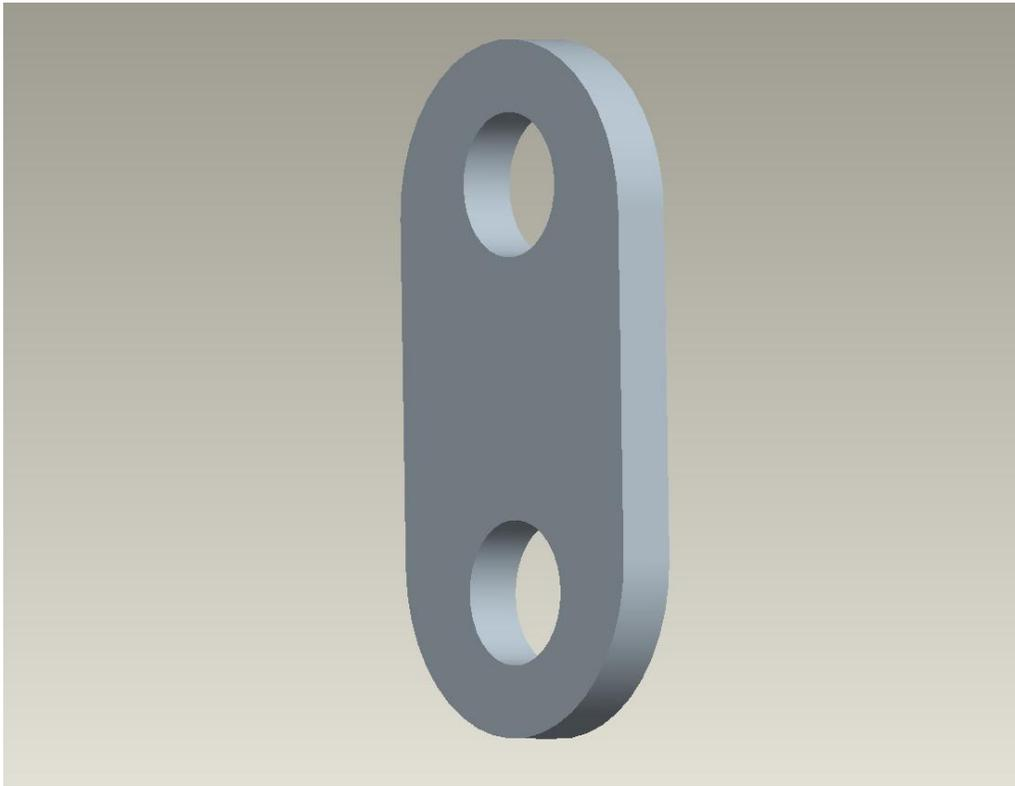
Figure D-4: Pro/E Model of the pivot allowing the leaf springs to deform
