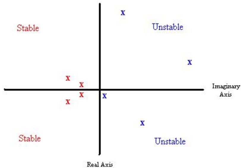
Figure 3-1: Eigen values plotted on the Imaginary and Real axes. The values in red demonstrate system stability while the values in blue demonstrate system instability.
