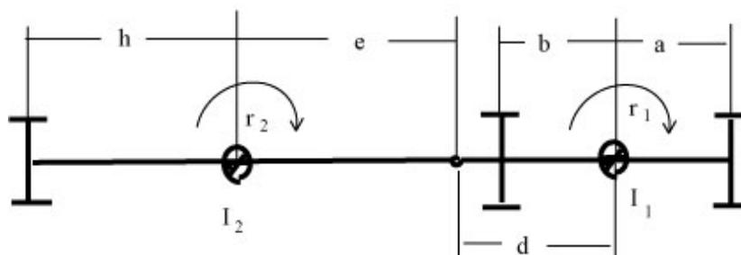
Figure 2-3: Critical distances and positive direction of yaw rate used in the derivation of equations of motion.
