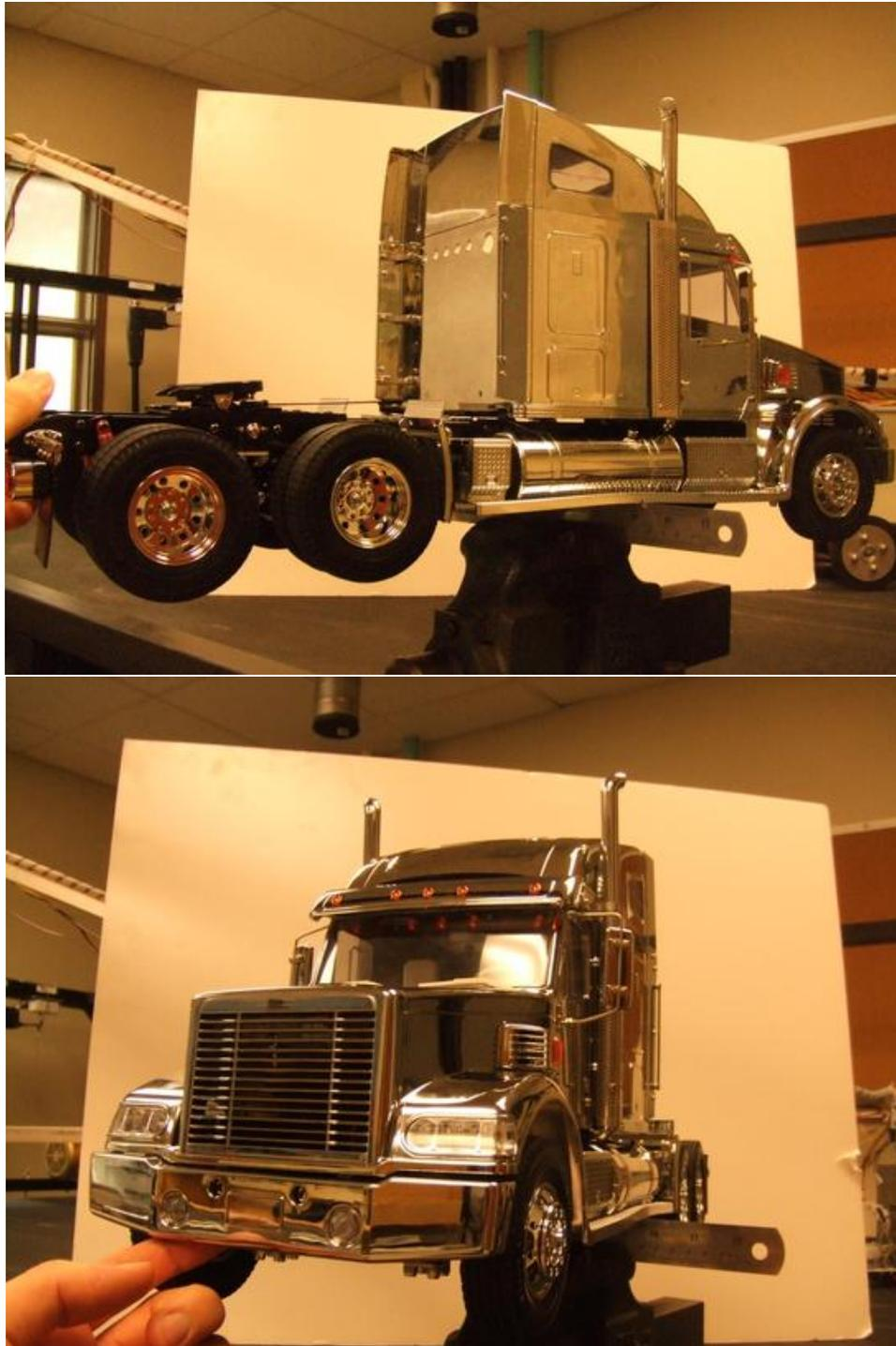
Figure 5-1: The scale tractor being balanced at different orientations to find the location of the center of gravity in the XY plane
