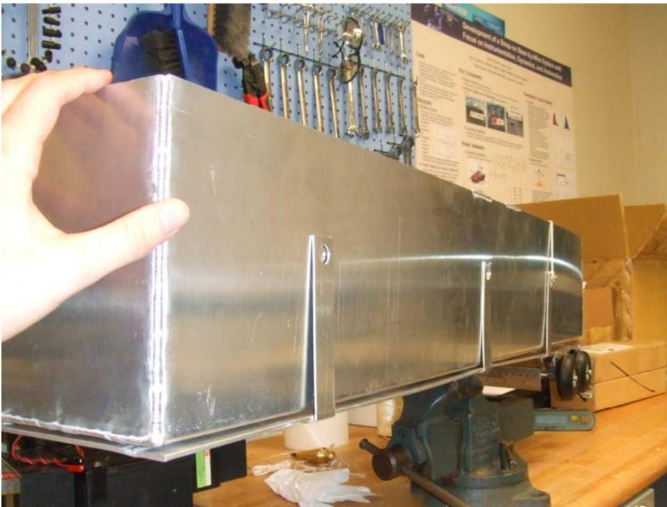
Figure 5-5: Estimating the location of the center of gravity in the XY plane for the combination container and chassis
