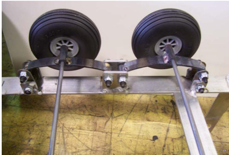
Figure 4-7: The two parallel axles on the trailer
