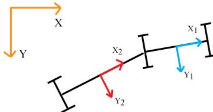
Figure 3-3: The global coordinates are shown in orange, while the body-fixed coordinates are shown in both blue and red.
