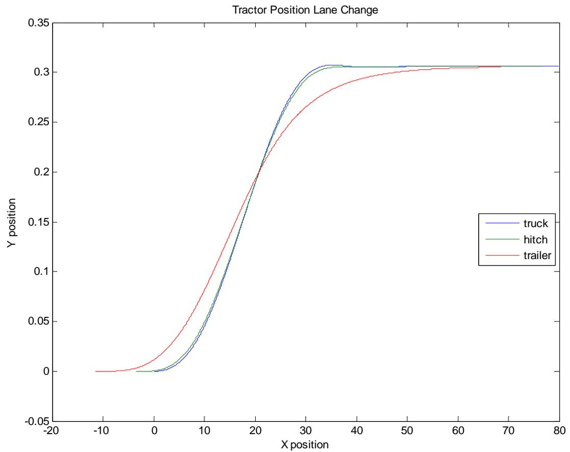
Figure B-1: The simulated response to a lane change maneuver at 4 m/s and a steering angle of 7 degrees = 0.1221 radians. The tractor trailer system behaves as expected. At low speeds, the trailer will track to the inside of the tractor during a turn.
