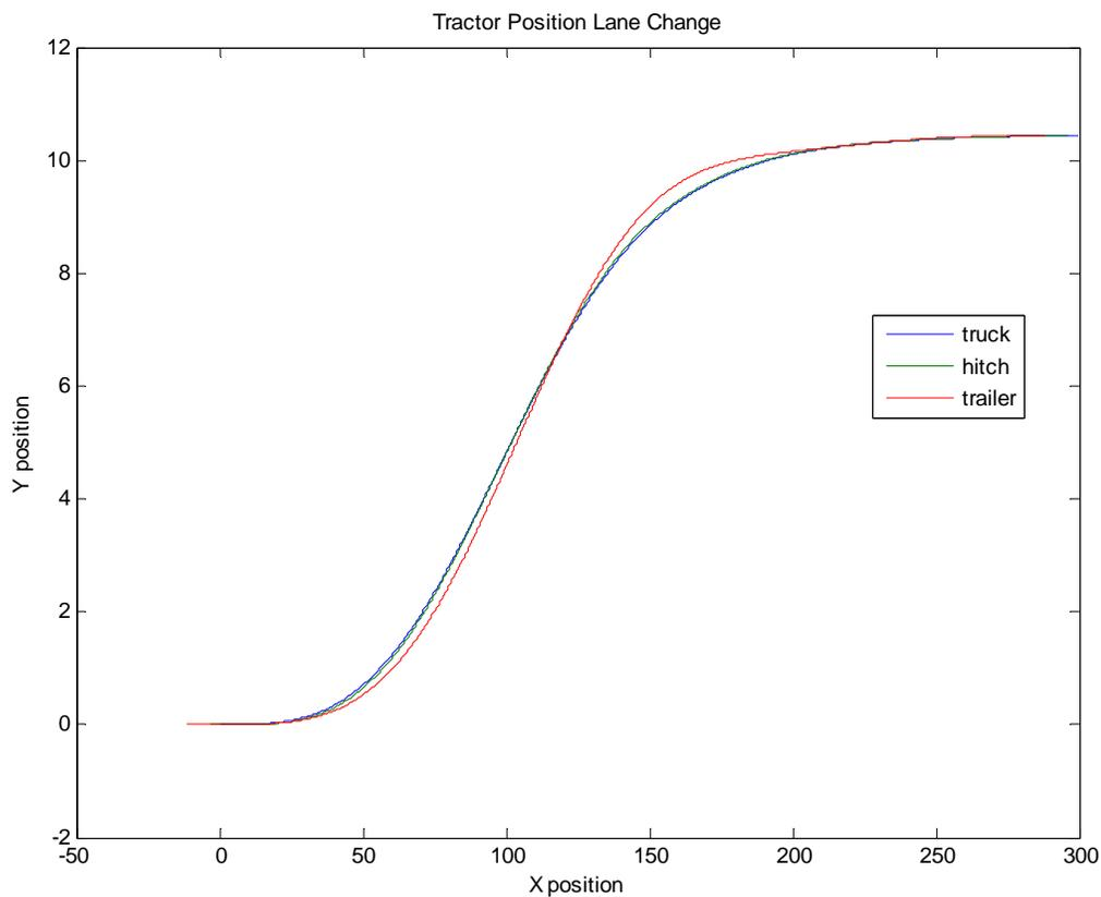
Figure B-2: The simulated response to a lane change maneuver at 15 m/s and a steering angle of 0.5 degrees = 0.0087 radians. The tractor trailer system again responds as expected. As the speed of the tractor trailer increases, the trailer will begin to follow a path similar to the truck.
