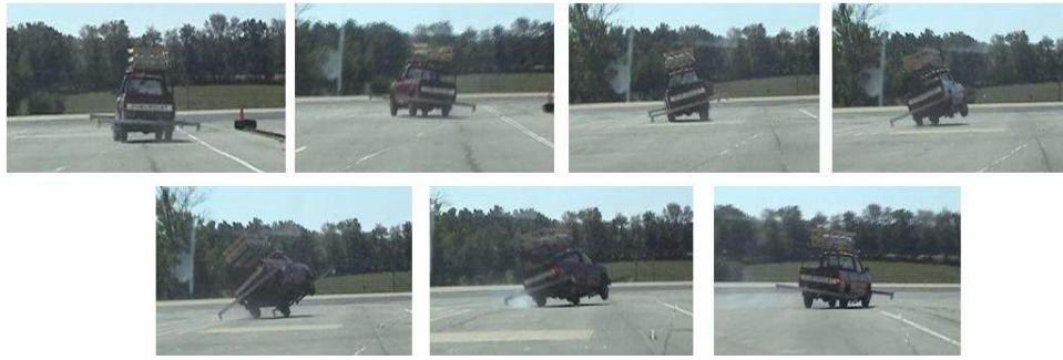
Figure 5.12: Snapshots of the truck during wheel liftoff.
